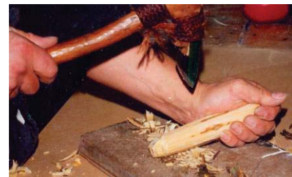
(Figure 2.10) Beveling the ends.
