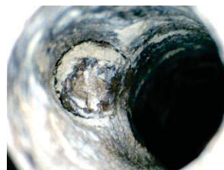
(Figure 4.18) Secondary pit. Note the white dust.
