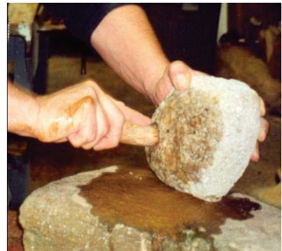
(Figure 4.9) Finishing with pumice.
