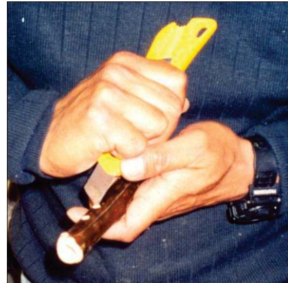
(Figure 2.18) Counter-sinking the wenewene.
