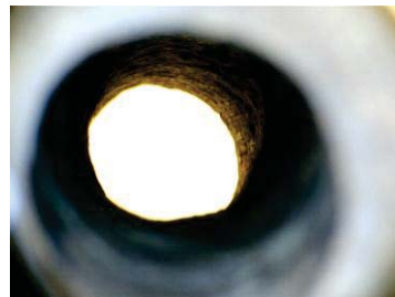
(Figure 4.17) Curvature of bore.
