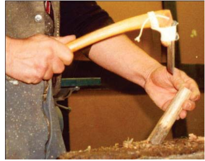
(Figure 4.7) Shaping with adze.
