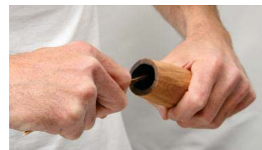
(Figure 5.9) Scraping the char from the bore.
