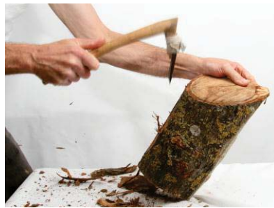
(Figure 4.28) Beginning to excavate the bore from a trunk.
