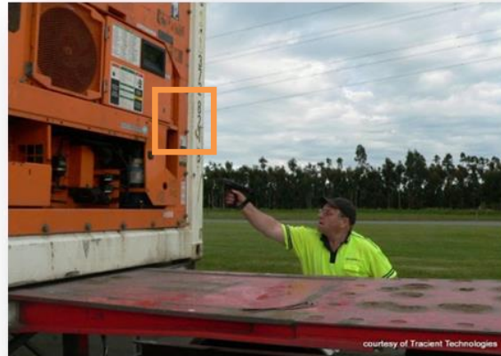
Figure 5.15 - Reading shipping container RFID tag ID at processor
