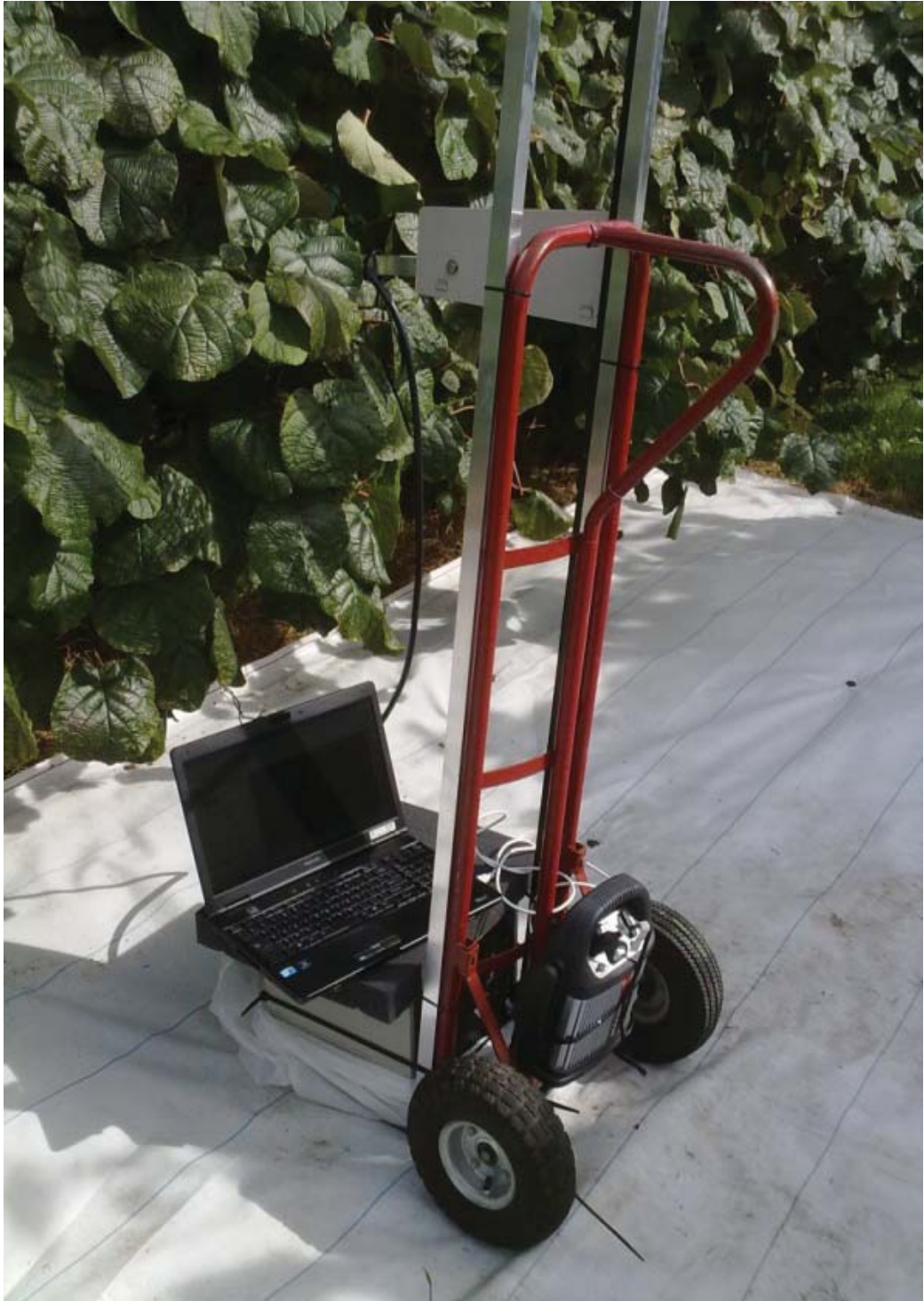
Figure 2-2: A photo taken in the kiwifruit orchard when we were doing the scan of lower canopy on 6 March 2012. The spectroradiometer was under the lap-top with the battery attached between the wheels. The sensor was bound with the arm to go through the canopy taking the scans.
