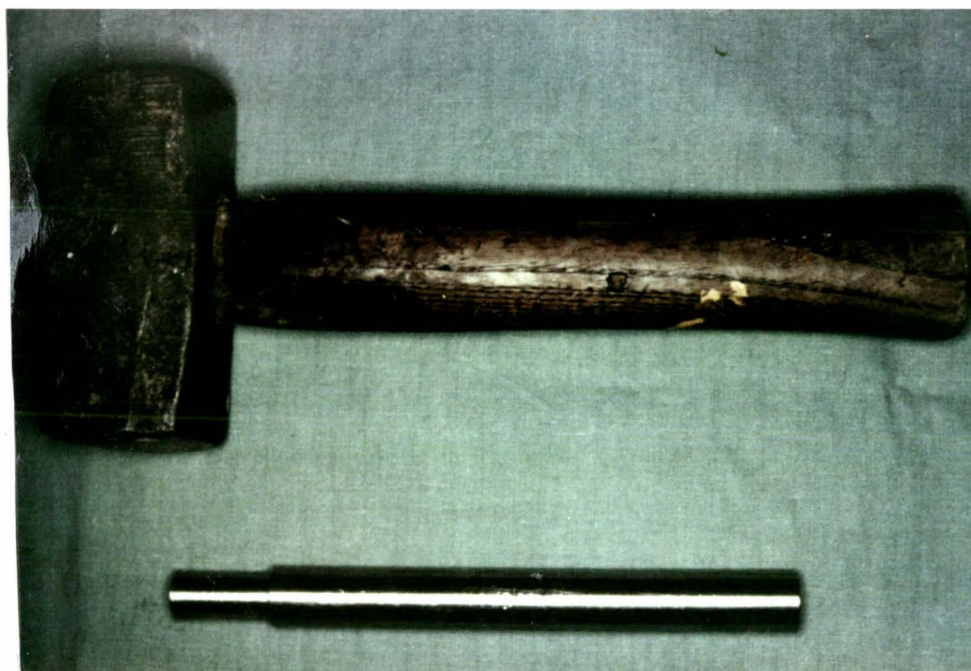
Figure 3.1 - Small hammer and steel rod and tube used for penetrative percussive stunning.
