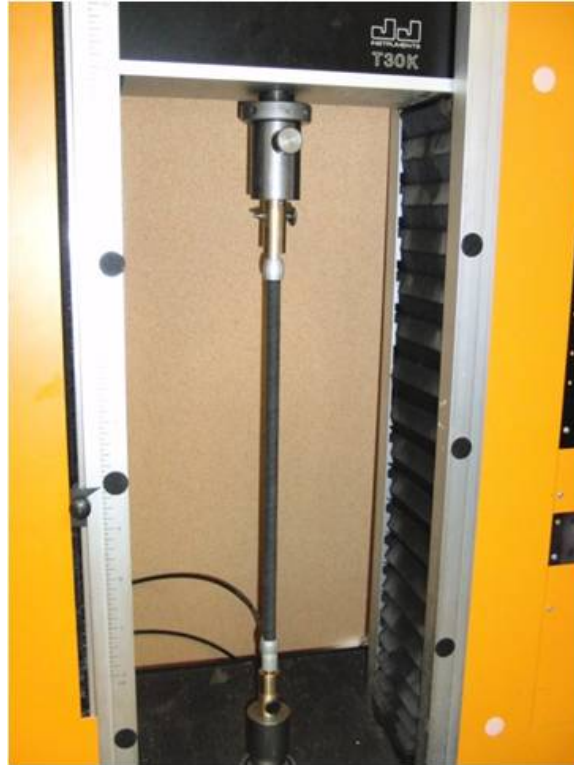
Figure 6-2: McKibben muscle's testing apparatus. Shown is a JJT30K tensionometer and a FESTA DMSP fluidic muscle.
