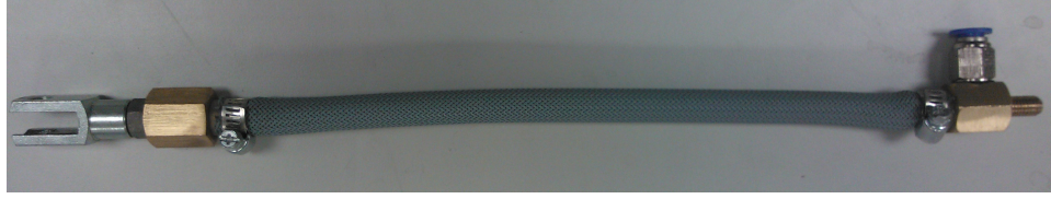
Figure 6-3: Fabricated pneumatic McKibben actuator used in this chapter, whose parameters have been experimentally determined, as discussed in subsequent sections. Here, the initial muscle length l_0 = 0.26 m and initial radius r_0 = 0.006 m.
