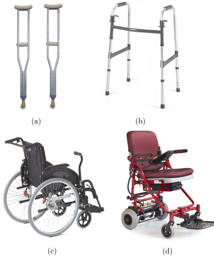
Figure 2-3: Examples of passive supportive assistive device examples. (a) Crutches; force is transferred from the upper chest to the ground via crutch's physical structure. (b) Walker frame; force is transferred from the hand grips to the frame's feet. (c) Invacare's Action3NG wheelchair [26]; torque, and subsequent displacement, is generated by force acting perpendicular to the wheel's rim. (d) Melrose Kiwi Concept Chair's powerchair [7]; controlled via a joystick, the power chair is a cost effective active support assistive device.
