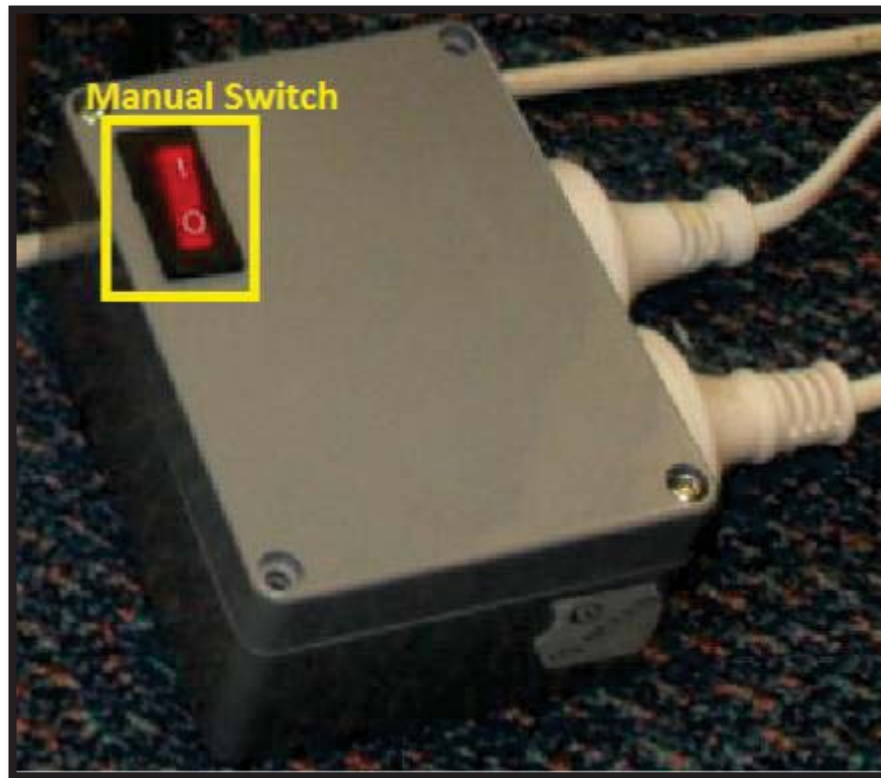
Figure 31: Hardware Unit showing the Manual Switch
