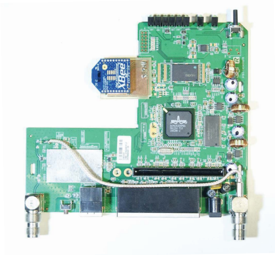
Figure 98 WRT54GL router with XBee Coordinator attached to serial port using fabricated PCB
