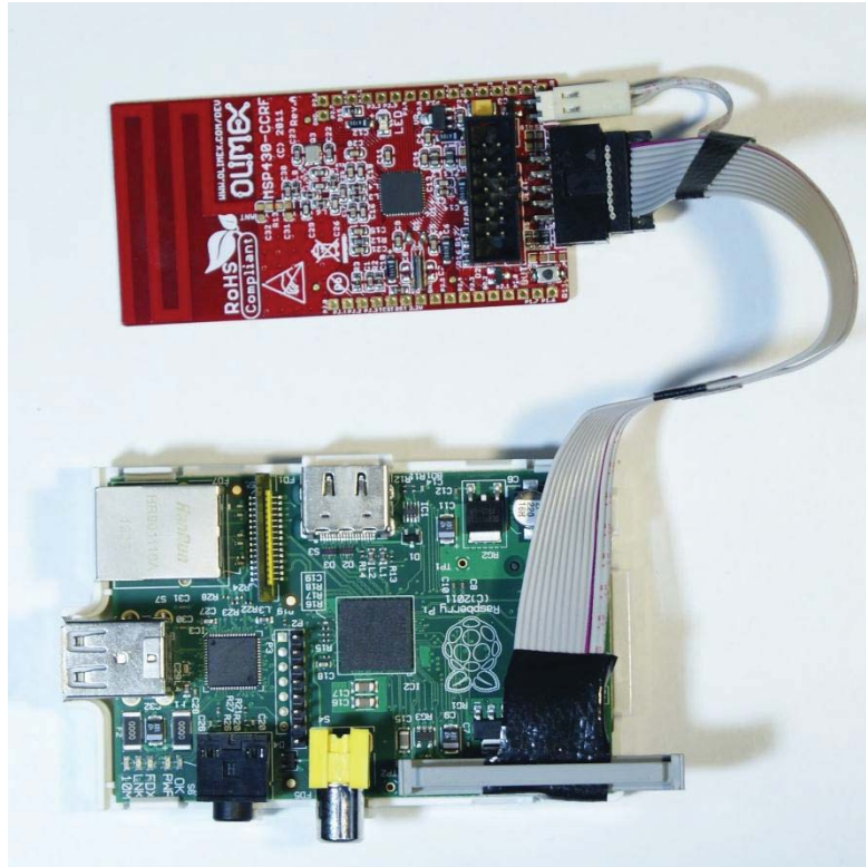
Figure 126 6LoWPAN gateway using the Raspberry PI connected to an Olimex CC-RF development board
