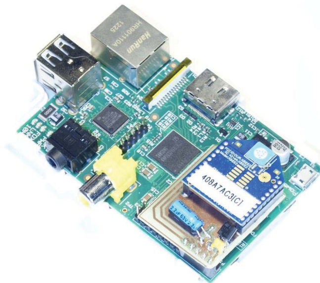
Figure 100 Raspberry PI with fabricated PCB for XBee coordinator to connect to serial port
