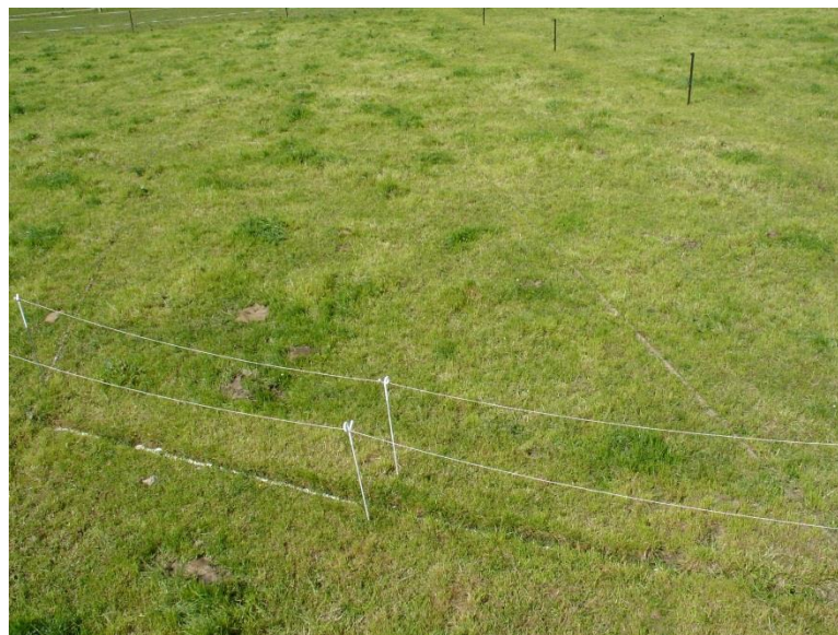
Plate 6.1: Example of a runoff plot photographed to observe spatial distribution of dung pats; runoff catching gutter is bottom centre, isolated by white electric fence standards.
