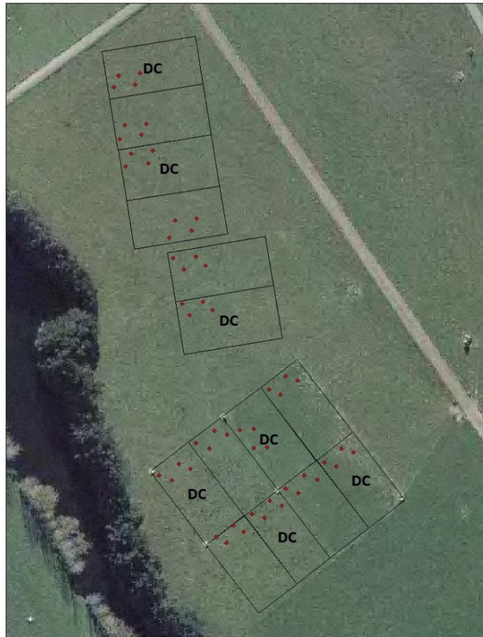
Plate 3.1: Layout of the fourteen ca. 850 m 2 , experimental plots (those marked with 'DC' denote Duration-controlled grazing plots, with the remainder being standard grazed plots; dots denote corners of 50 m 2 runoff plots)
