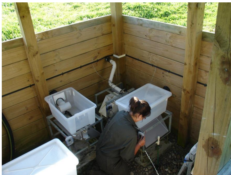
Plate 4.1: Individual tipping buckets and collection area for drainage and runoff water.
