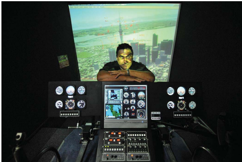
Figure 6-7. Completed ARHT PCATD
