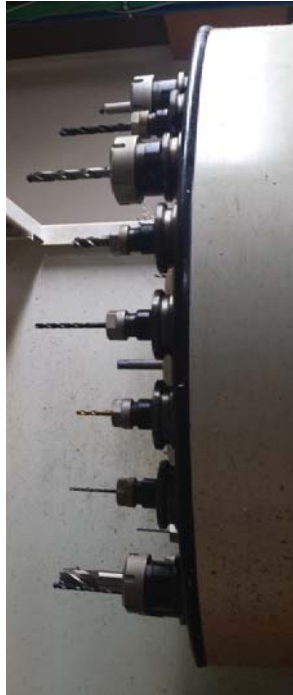
Fig. 5.4 - Automatic tool changer for the Acumen 500 CNC Machining Centre
