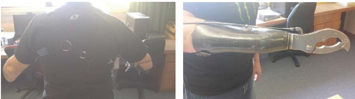
Fig. 4.21 - Hook Prosthetic Actuation Harness (Left), Hook being Closed by Harness (Right)
