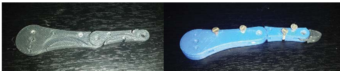
Fig. 4.4 - 3D Printed Finger Revision 1 (Left), 3D Printed Finger Revision 2 (Right)
