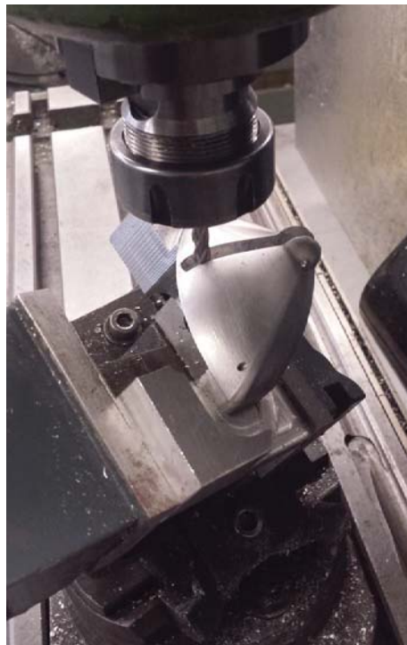
Fig. 5.14 - Guide Channel Manufacture
