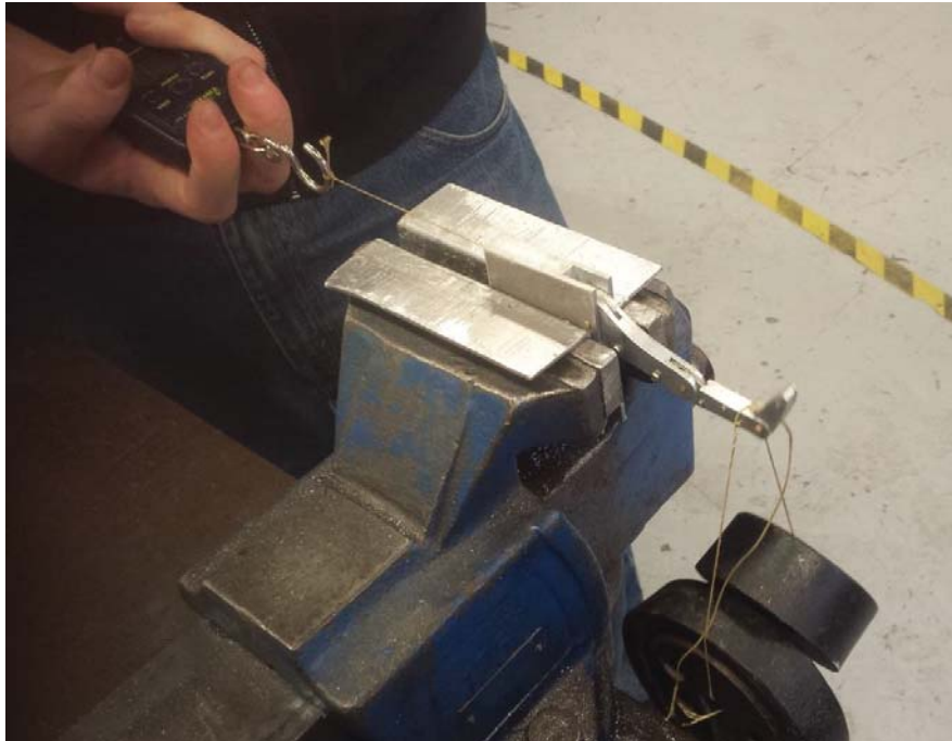
Fig. 4.8 - Weight Lift tests of Prototype Finger Worst Case Scenario
