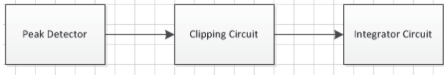
Fig. 6.27 - MAV Implementation 3 Block Diagram
