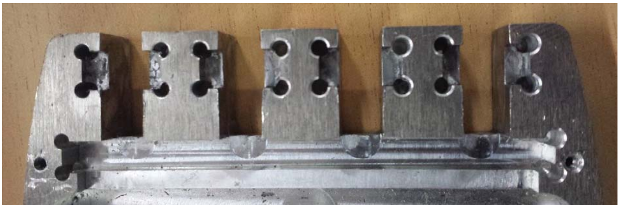
Fig. 5.9 - Designed Corners (Above) Vs Machined Corners (Below)
