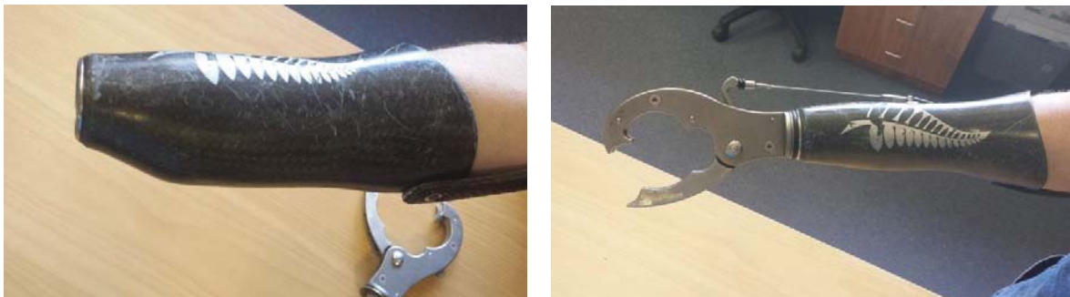
Fig. 4.20 - Current Carbon Socket (Left), Socket with Hook Attached (Right)
