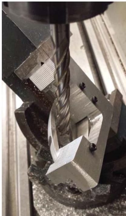
Fig. 5.13 - Long Shank End mill and Angle vice Setup
