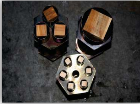
Figure 6.1: Top view of pyrolyser wood holders
