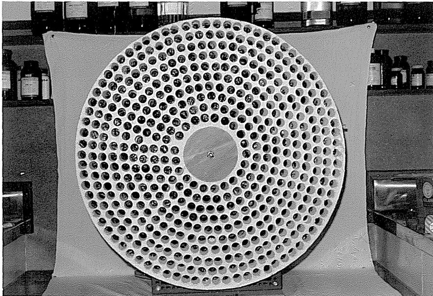
Figure 8. Rotating wheel for coleoptile bioassays
