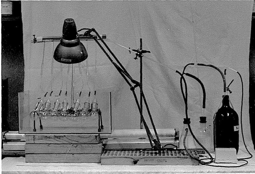
Figure 10. Apparatus used for Commelina communis epidermal strip bioassay. Shown from right to left are the air pump, CO<sub>2</sub> scrubber, pressure head regulator, washing bottle, and combined manifold and incubating flask holder immersed in a glass water bath. Above the bath is the incandescent light source and below, the fluorescent tubes.
