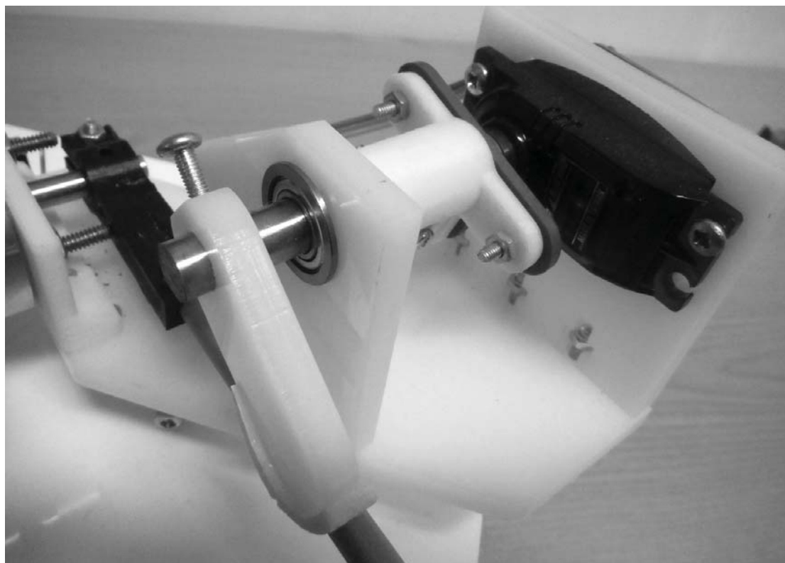
FIGURE 5.10: A detail of Nudge’s cam-based solenoid height stop. The miniature servomotor, shown at right, rotates the shaft-mounted cam, changing the drumstick’s at-rest height.
