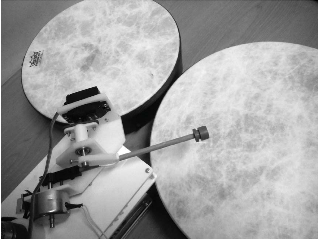
FIGURE 5.6: Nudge with multiple drums: by rotating its motorised turntable, Nudge can move to strike multiple objects within its workspace.
