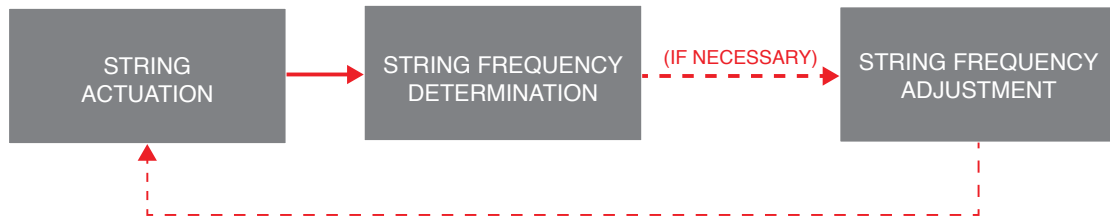
FIGURE 6.2: A typical self-tuning procedure: upon actuation, the string’s frequency is measured and, if necessary, the string’s tension is adjusted. After adjustment, the string is again actuated and measured.
