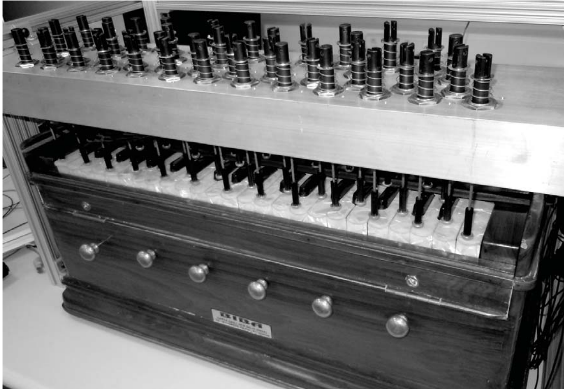
FIGURE 4.3: Kritaanjli’s keyboard player: each of the 44 solenoid actuators is positioned above a key. Upon actuation, the solenoid’s plunger extension depresses its key. The width of the solenoids necessitated their staggered placement above the keyboard.
