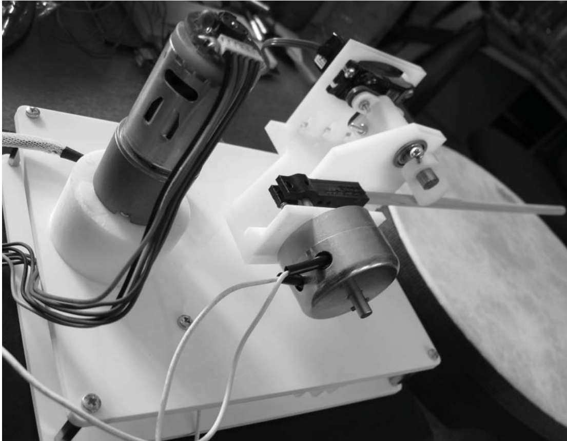
FIGURE 5.1: Nudge: at left is the DC servomotor connected to the turntable. The turntable pivots the solenoid-mounted drumstick (right) and its accompanying stick height stop.
