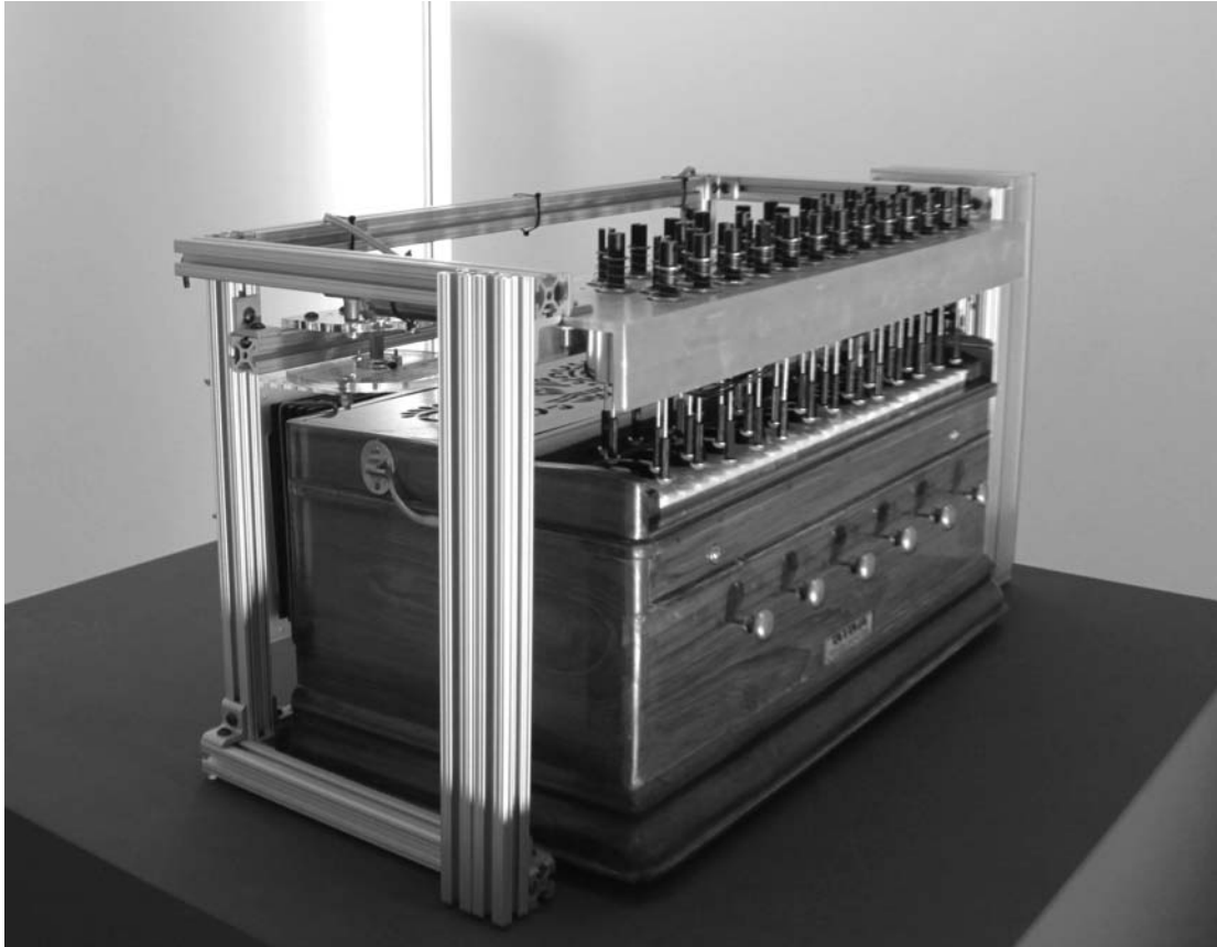
FIGURE 4.2: Kritaanjli's chassis and subassemblies. The extruded t-slot aluminium chassis forms a cage around the harmonium, to which are attached the actuators (centre and upper left) and electronics (right).
