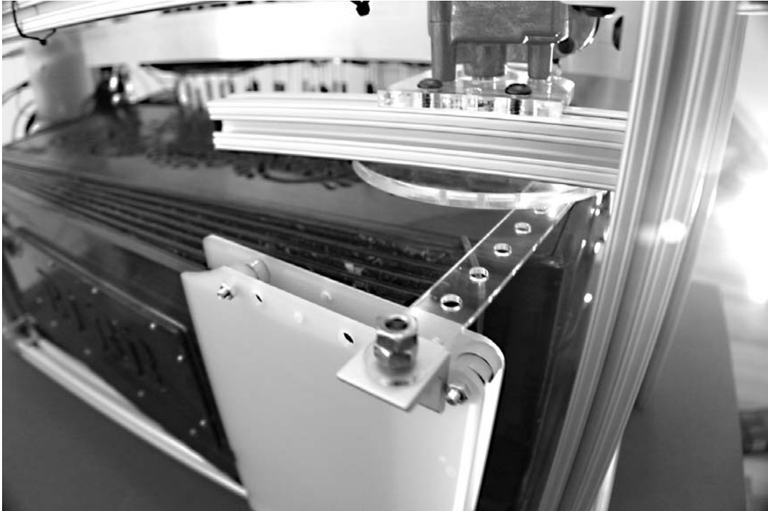
FIGURE 4.7: Kritaanjli's bellows pumping mechanism clamped to the harmonium's bellows.
