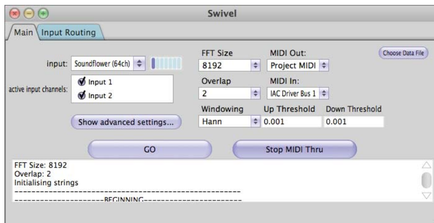
FIGURE 6.6: SwivelSelfTune’s GUI: FFT settings, string characterisation files, and MIDI and audio input and output routing can be specified by the user. Once the string is tuned, the user can switch into “running mode” by pressing the “Start MIDI Thru” button.
