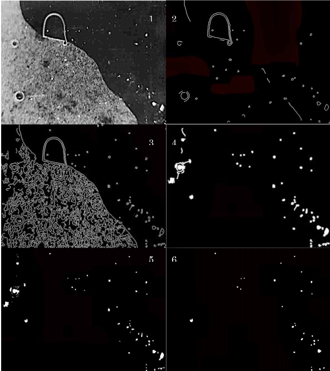
Figure 6-3: Images of segmentation sequence. Top left to bottom right are: 1. original image, with the wax seal covering the left half 2. edges using the original image to calculate threshold – note missing pollen 3. edges using background image to calculate threshold 4. edges dilated, filled and the borders cleared 5. erosion brings blobs to original object size and smooths edges 6. final objects are found with some objects removed by various tests described in the text
