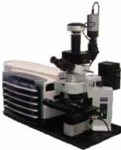
Figure 8-6: Olympus BX61. A commercial automatic microscope with digital camera, auto-focus, XY stage movement and slide stacker valued at about $AUS150,000
