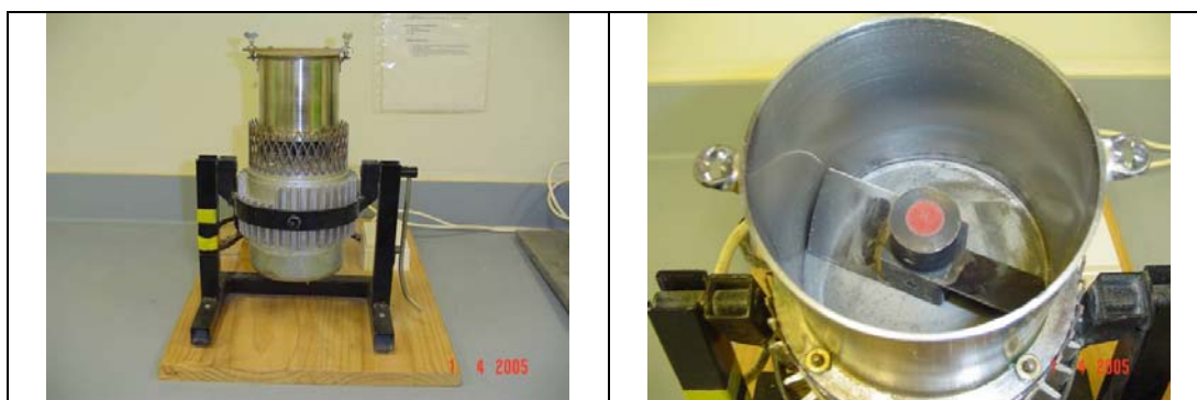
Fig 3.14: The breakage tester (Developed by the Crop and Food Research, Ltd.)
