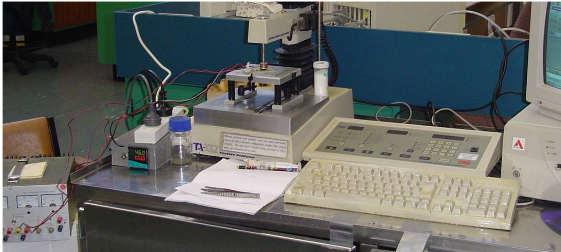
Fig 3.19: The combination of a heating unit and the Food Texture Analyzer
