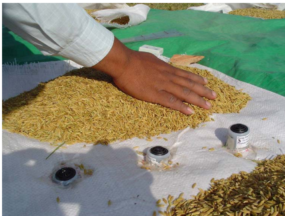
Fig 3.5: Positions of the TinyTag/ Tinytalk relative humidity sensors
