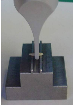
Fig 3.13: Three-point bending cell (Made by the ITE workshop)
