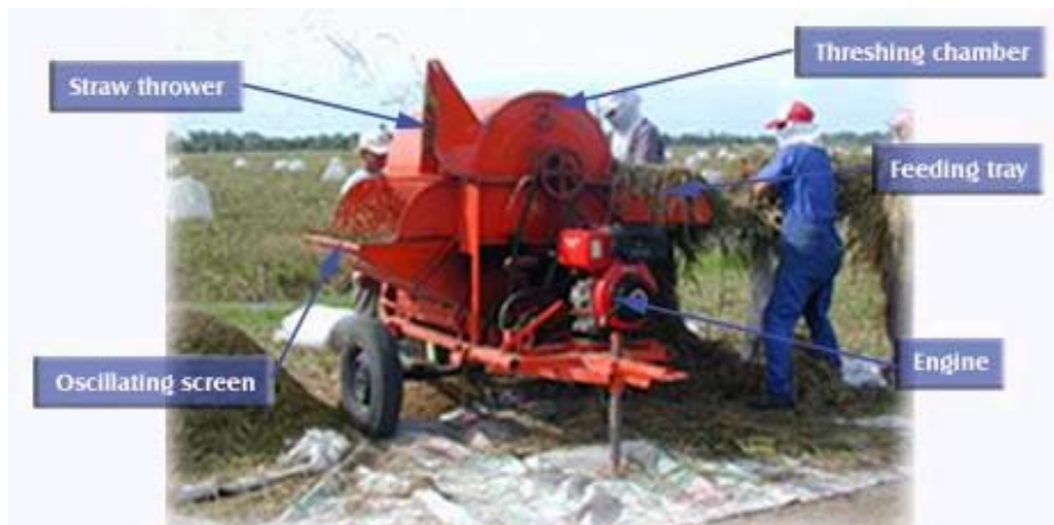
Fig 2.13: Axial-flow rice thresher (Source: Cruz and Havard, 1994)
