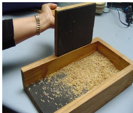
Fig 3.15: Grain dehusking tool (developed by the Crop and Food Research, Ltd.)
