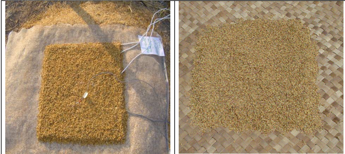
Fig 3.12: The grain samples being dried on nylon net spread on husk and on the mat spread directly on soil
