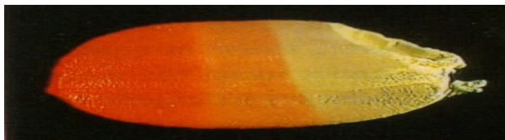
Fig 2.12: Fissures in a rice kernel as seen through a red light filter (Source: IRRI, 2002b)
