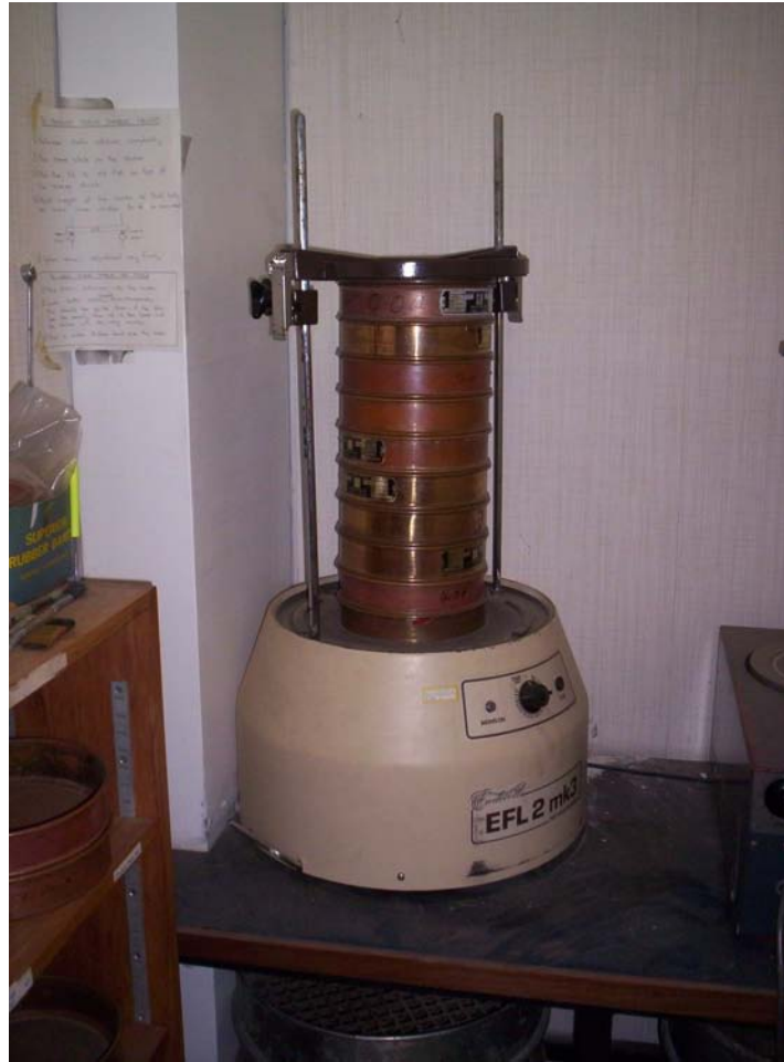
Figure 6.4 A sieve shaker (EFL 2 mk3). The sediments were air dried and sieved at half-phi intervals from 0.5 \phi to > 4 \phi .
