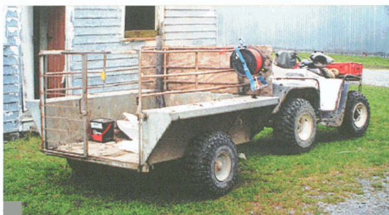
Figure 1.5 Early two-wheeled drive 250cc model – very easy to steer by comparison to heavier more recent 4WD quadbikes
