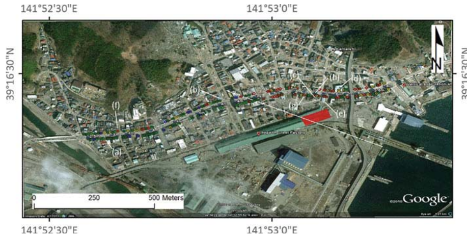
Fig. 3 Damage survey in Kamaishi City with individual buildings plotted to show construction and damage level. Construction type is indicated by shape, EEFIT tsunami damage level by colour: Diamonds denote timber frame; squares denote RC; circles denote steel frame. Blue denotes D0, green denotes D1, yellow denotes D2, orange denotes D3, red denotes D4. Inundation depths, the collapsed section of Nippon Steel Factory building (red polygon), and vertical evacuation building are also shown. White letters show the position of buildings shown in Fig. 4
