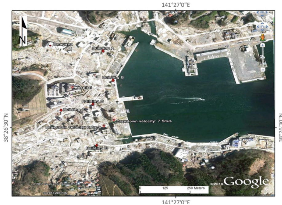
Fig. 16 Satellite image of the harbour in Onagawa Town, indicating the (i) final locations of overturned RC and steel frame buildings (blue points, marked with building tag A–E) as observed by EEFIT; (ii) the track of building movement from the original position indicated by arrows (Tokimatsu et al. 2011); and (iii) positions of two velocity estimations made for return flow velocity using video footage
