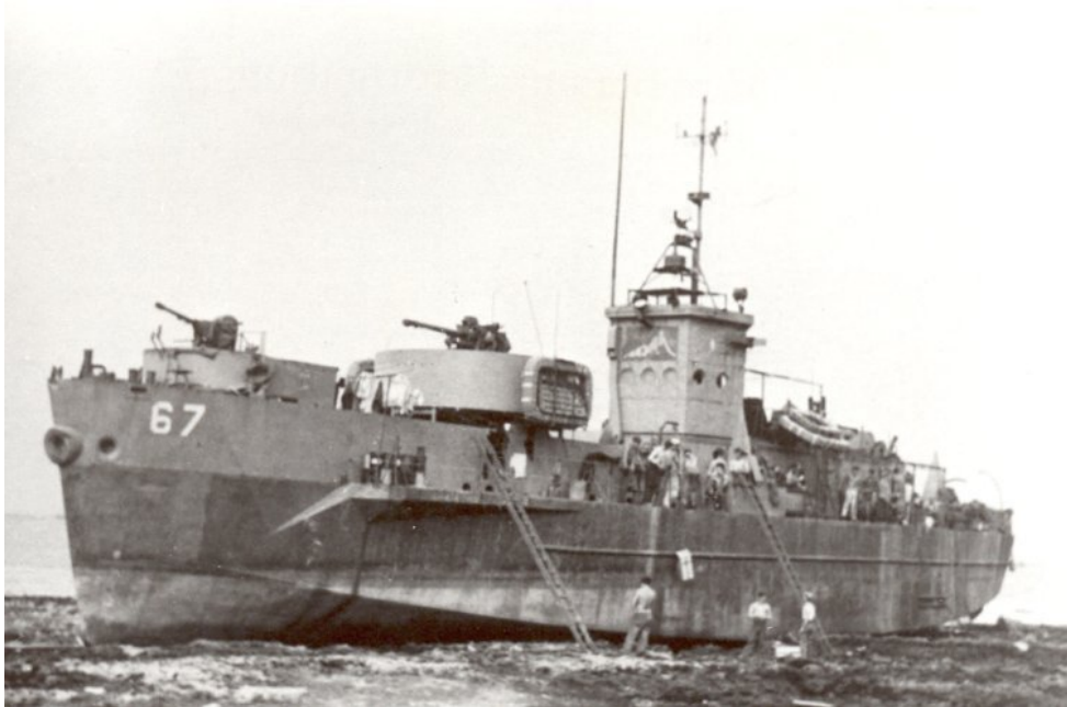
Image 13: A late war picture of LCI(G) 67 stranded on a beach at Okinawa in 1945 – the 3-inch gun and at least one of the 40mm Bofors may be seen, as well as the landing craft’s emblem on the superstructure which appears to be a mermaid. (Source: NavSource Online: Amphibious Photo Archive, http://www.navsource.org/archives/10/15/150067.htm .)
