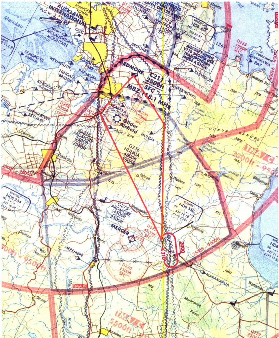
Figure 40. Aeronautical Map of South Auckland. (The red lines show the departure and arrival tracks required between Ardmore Airfield and the Surrey NDB. The Surrey NDB holding pattern is also highlighted in red).
