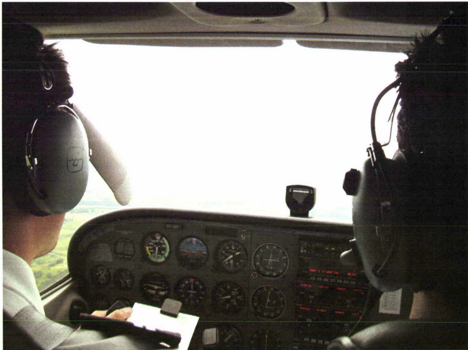
Figure 18. Student Wearing IFR Hood While Flying on Instruments.
