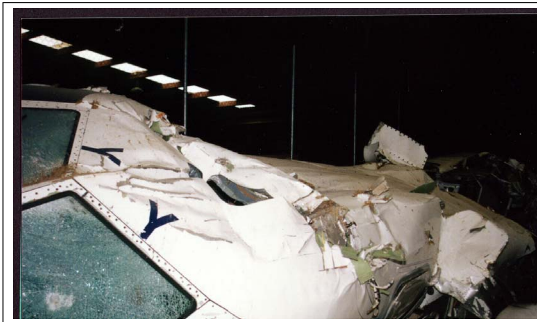
Figure 39. View from front of fuselage, showing crush lines and ingrained dirt.
