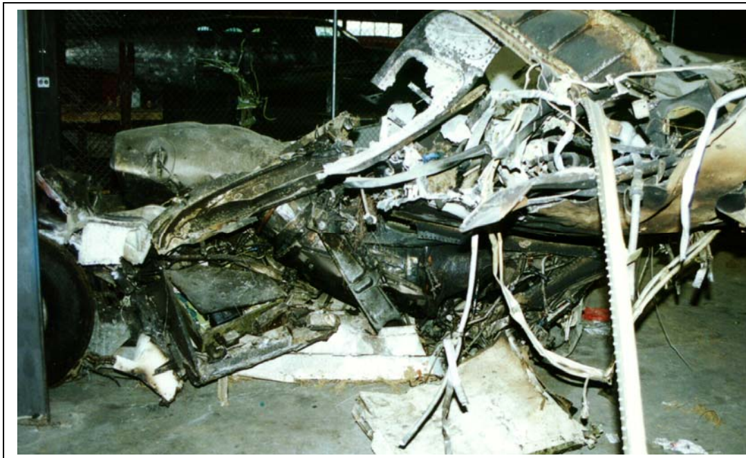
Figure 43. Starboard wing outboard of nacelle. Downward deflection of lower surface; spar web pulled away from spar caps. There has been no loading of the web in shear.
