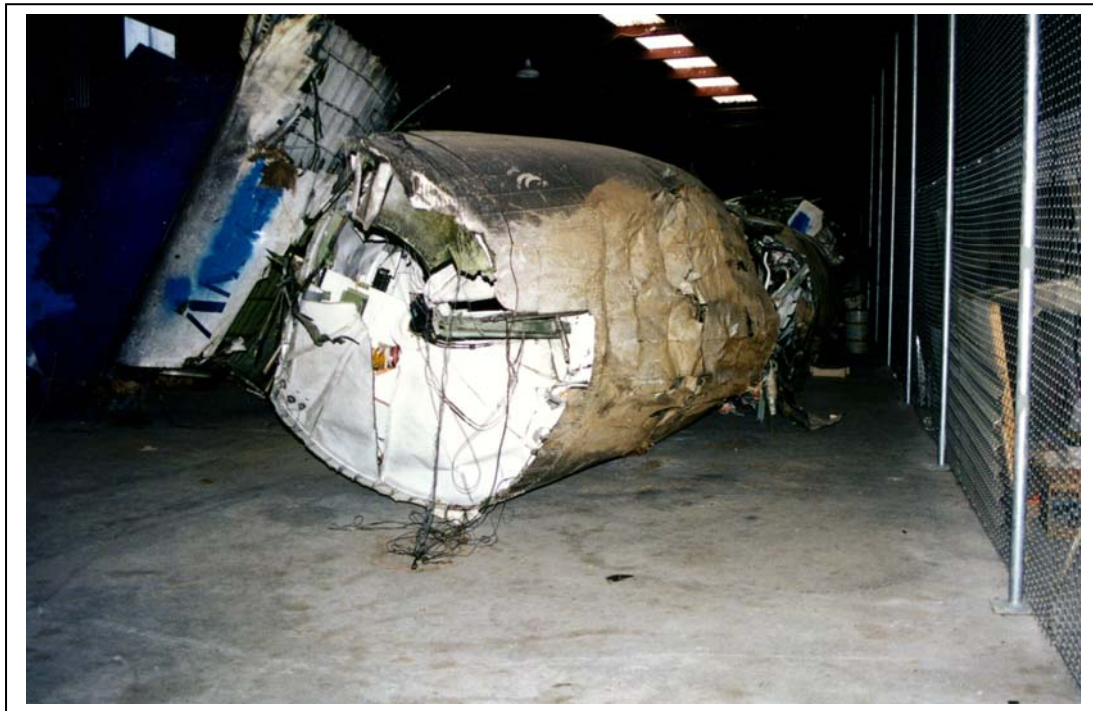
Figure 42. View from bottom rear of fuselage. Impact damage is ahead of rear bulkhead. Note flattening at top of rear fuselage.
