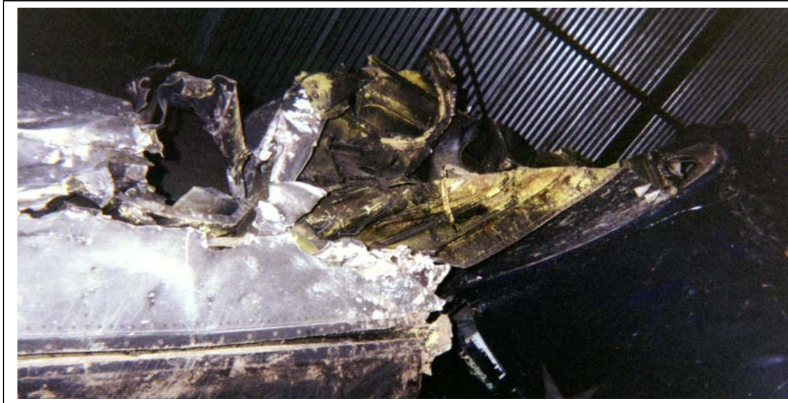
Figure 44. Damage to upper skin of starboard tailplane. The square hole has extensive sooting inside; the deflection damage has very little sooting. Soot deposits around rivets are fairly even, suggesting static fire.
