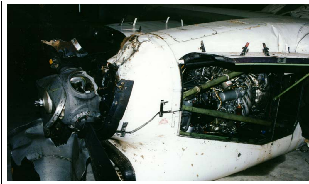
Figure 41. Left engine nacelle, showing lack of damage to underside, and inverted ground contact. Damage to the propeller shows that it was in this position, and rotating, when the nacelle struck the ground.
