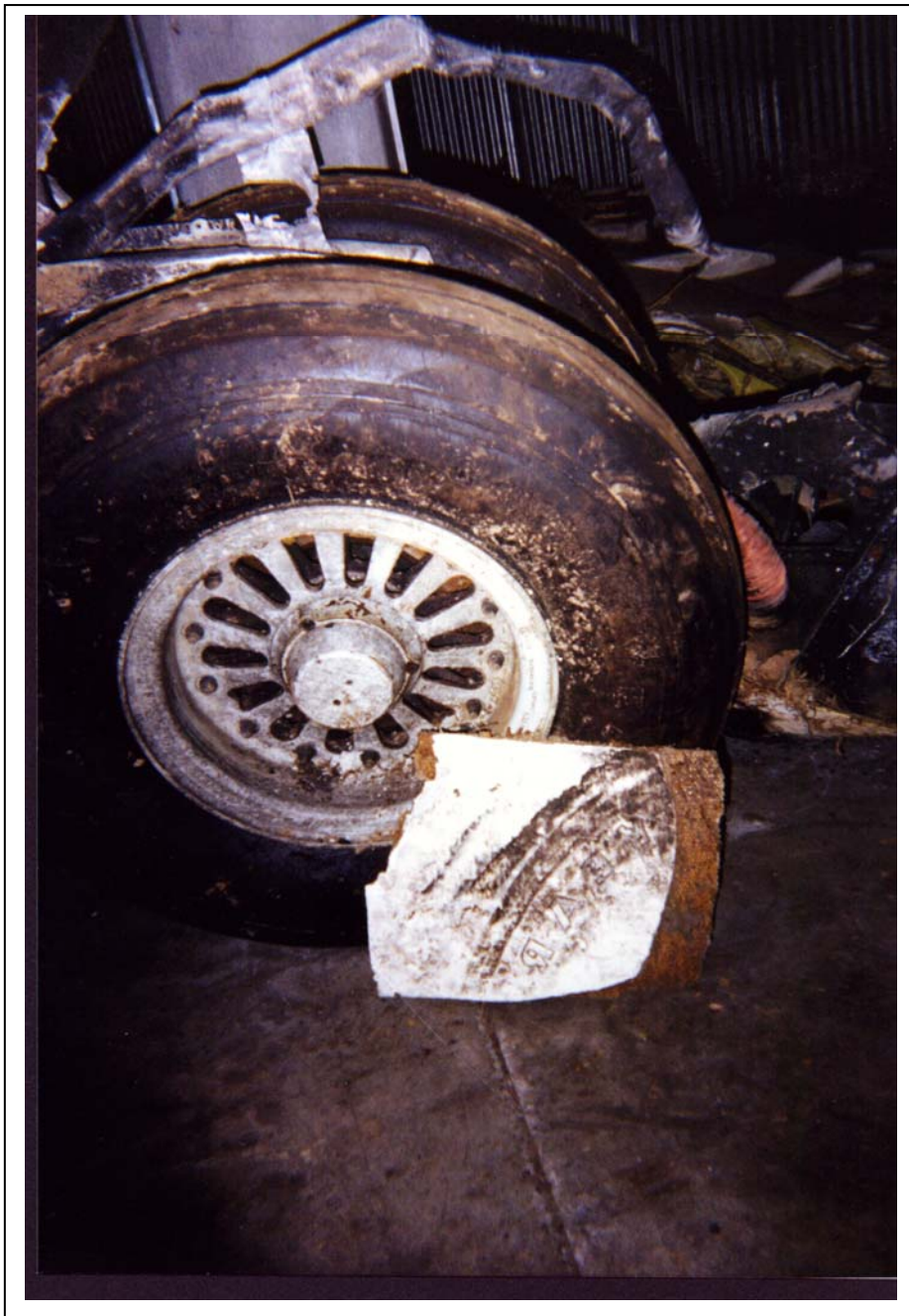
Figure 38. Witness mark on right hand undercarriage door.
