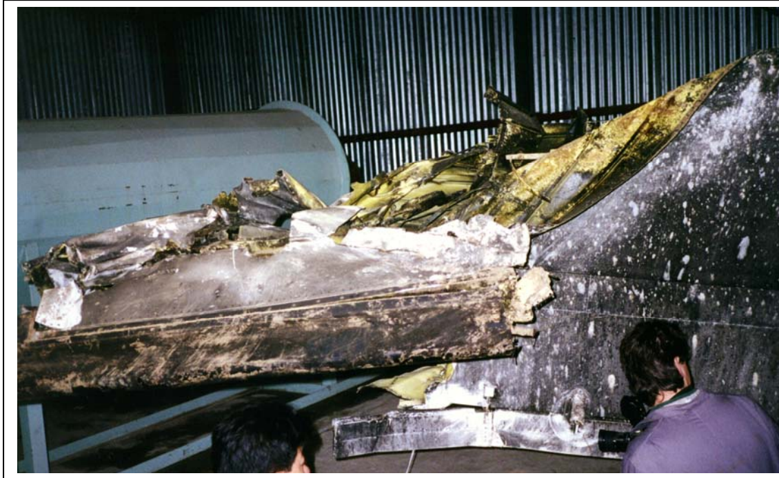
Figure 45. Damage to leading edge of fin and upper surface of tailplane. There was no corresponding damage on the outer portion of the right wing.
