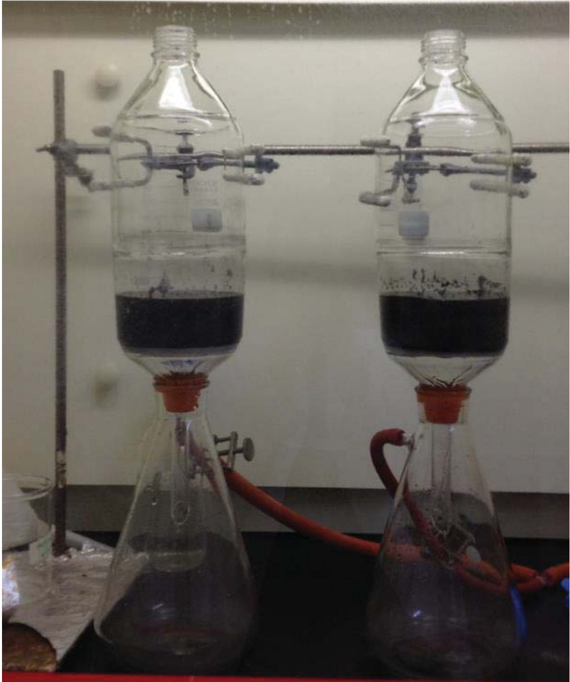
Figure 3-2 Charcoal media and vacuum system utilised to separate sugars
