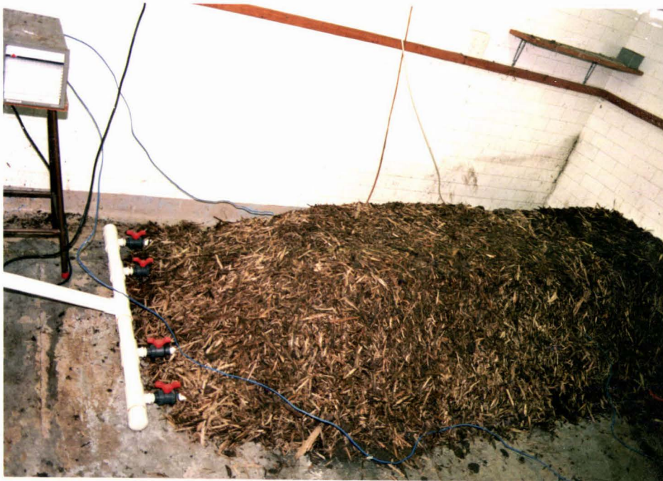
PLATE 3.4: Experimental aerated static compost pile comprised of woodchips and secondary sewage sludge. Note manifold for air distribution. Twelve thermocouples (not presented in this photograph) allowed the recording of temperatures throughout the pile.
