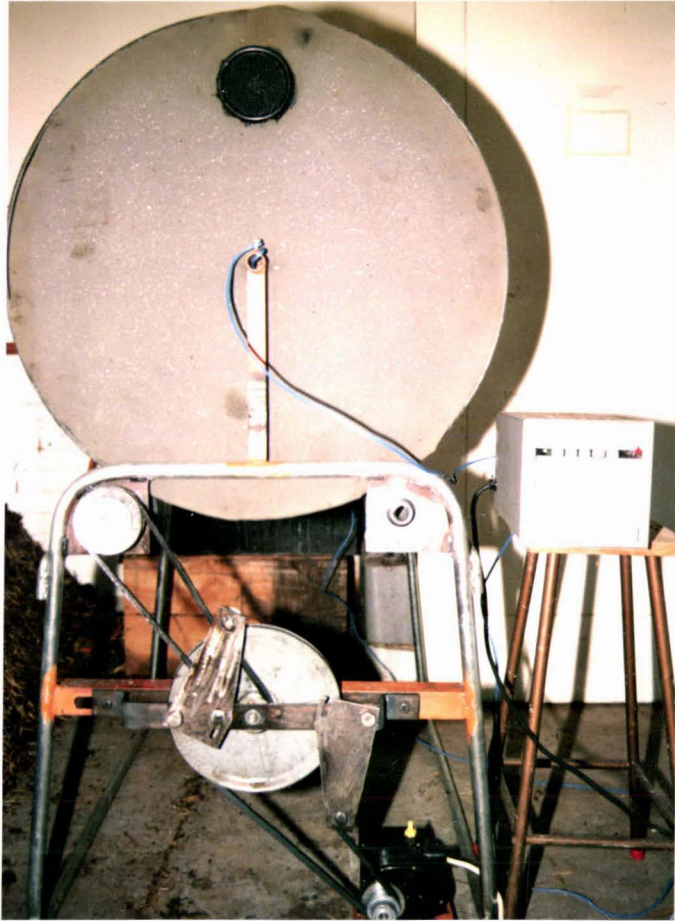
PLATE 3.3: Compost tumbler for tumbling and composting woodchips and secondary sewage sludge. Temperature recorder and thermocouples are in place.
