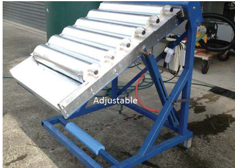
Figure 3-6, Demonstration of flow slope adjustable of the project prototype
