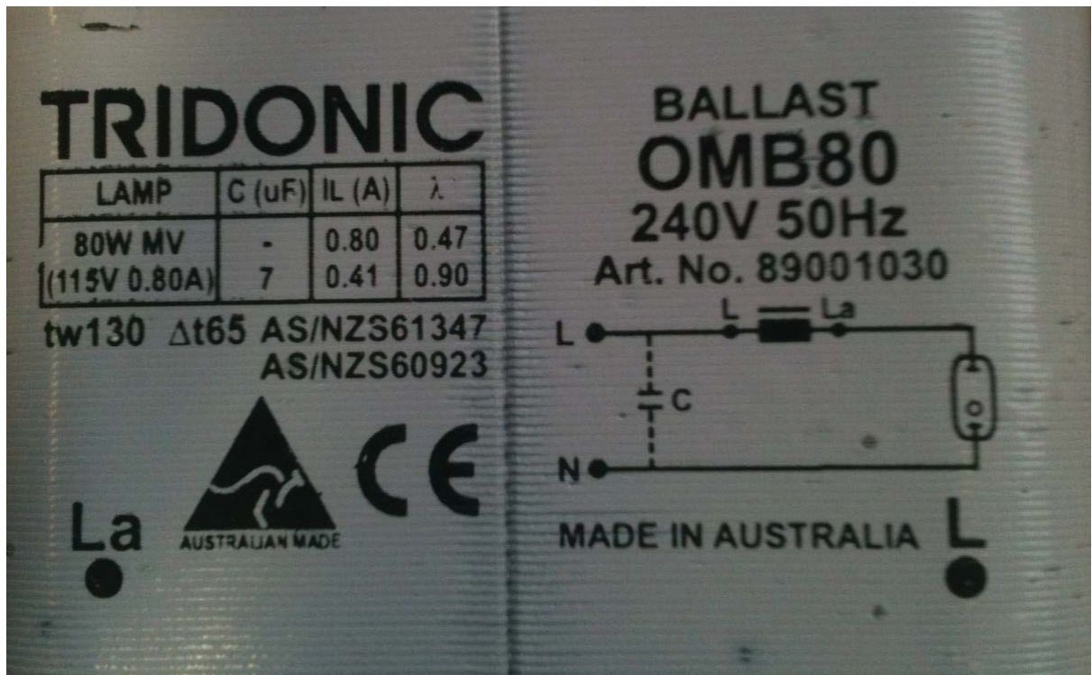
Figure A-7-8, information of the ballast used in the project
