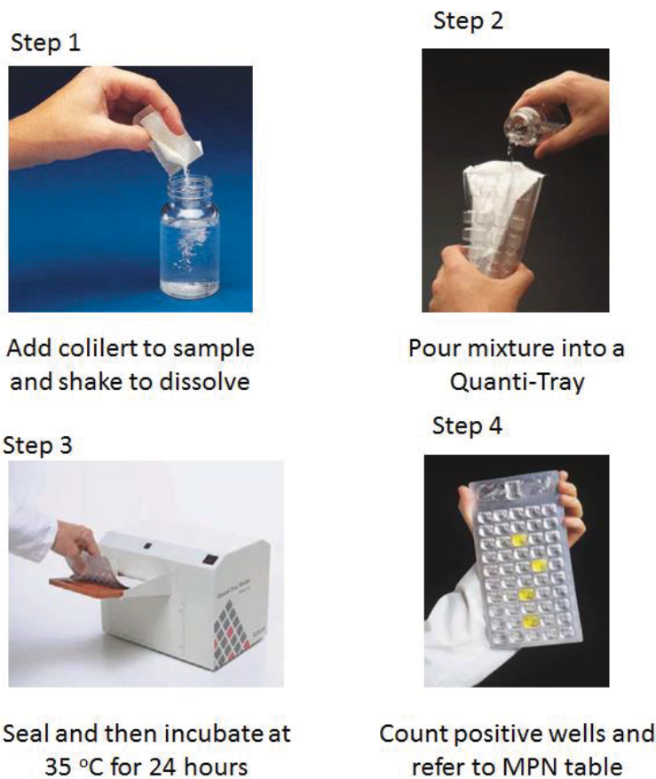
Figure 3-19, Colilert test procedure (adapted from IDEXX Laboratories, 2013)
