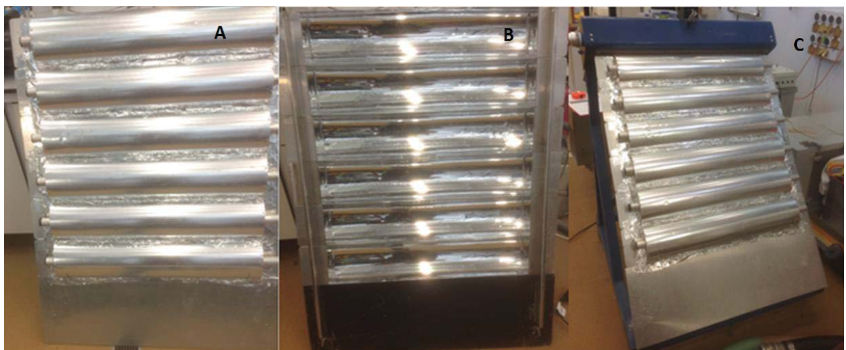
Figure 3-7, Parabola reflector (A: top of reflector; B: underside of the reflector; C: reflector on the project prototype)
