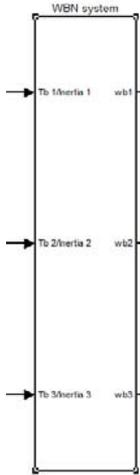
This block represents the angular velocity of the satellite, we can see that torque from magnetic coils is one of the main components for this block of the system, and it's logical as the angular velocity changes with amount of torque applied.
