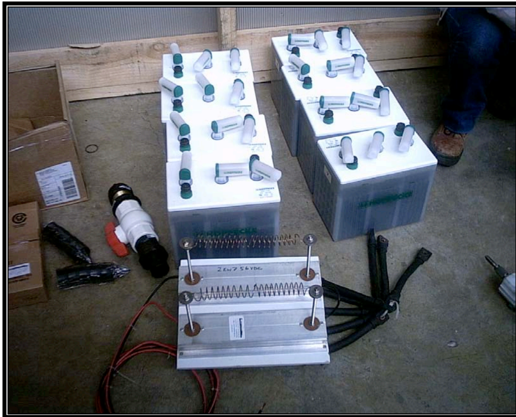
Figure 20 System components including pipe fittings(left), dump load(front) Battery links (black objects front right) and batteries (top of picture).
