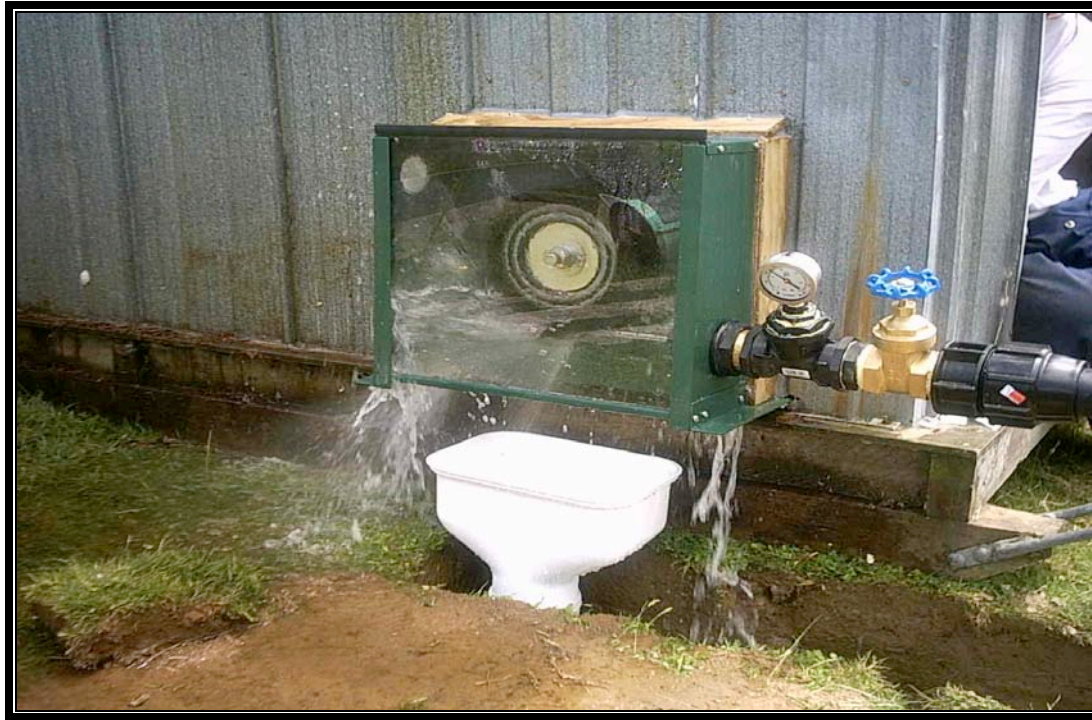
Figure 16 Turbine undergoing initial testing
