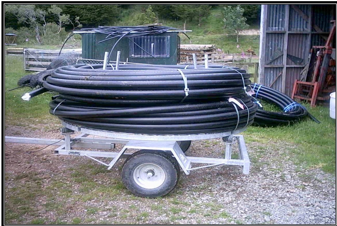
Figure 14 63mm MDPE agricultural pipe used for the “Penstock”
