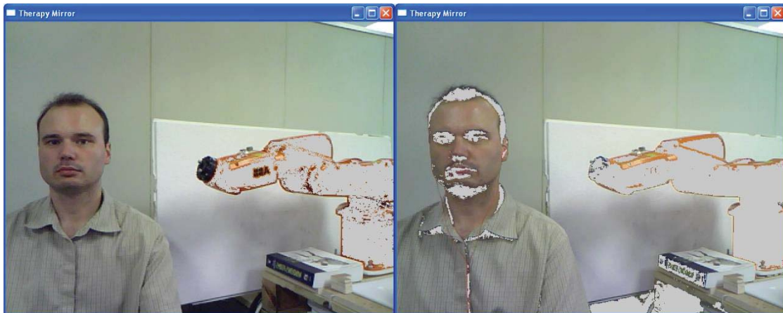
Figure 4.4 - A demonstration of chroma key applied with edge detection implementation (left) and without edge detection implementation (right)
