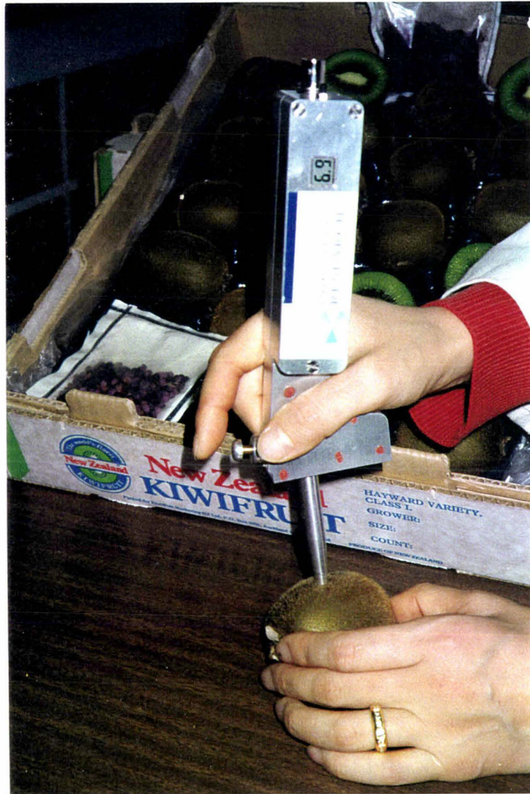
Plate 2.2 – The ‘Kiwifirm’, device used for measuring fruit firmness non-destructively.
