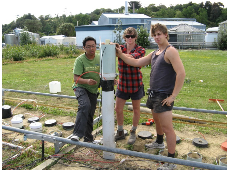
Picture 4.2. Soil column with TDR installed
