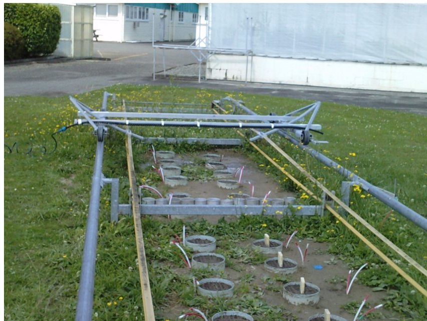
Picture 4.3. Lateral drip irrigation machine used in the experiment
