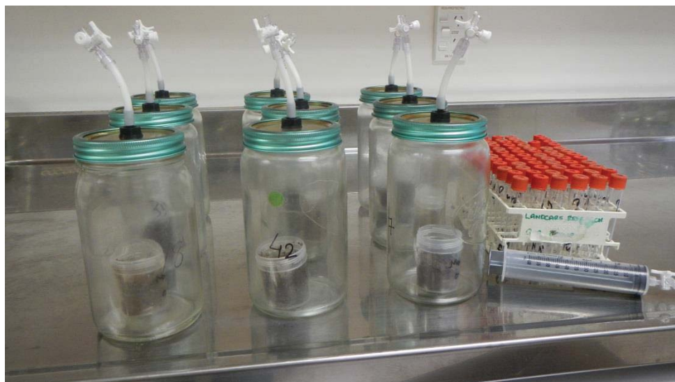
Figure 6.1 Incubation of soil samples in jars for gas analysis.
