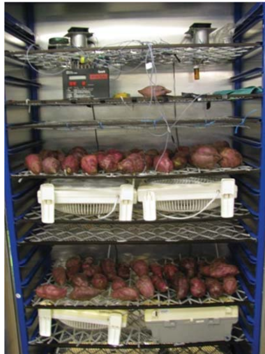
Figure 4.3: Cabinet used for water vapour permeance measurements
