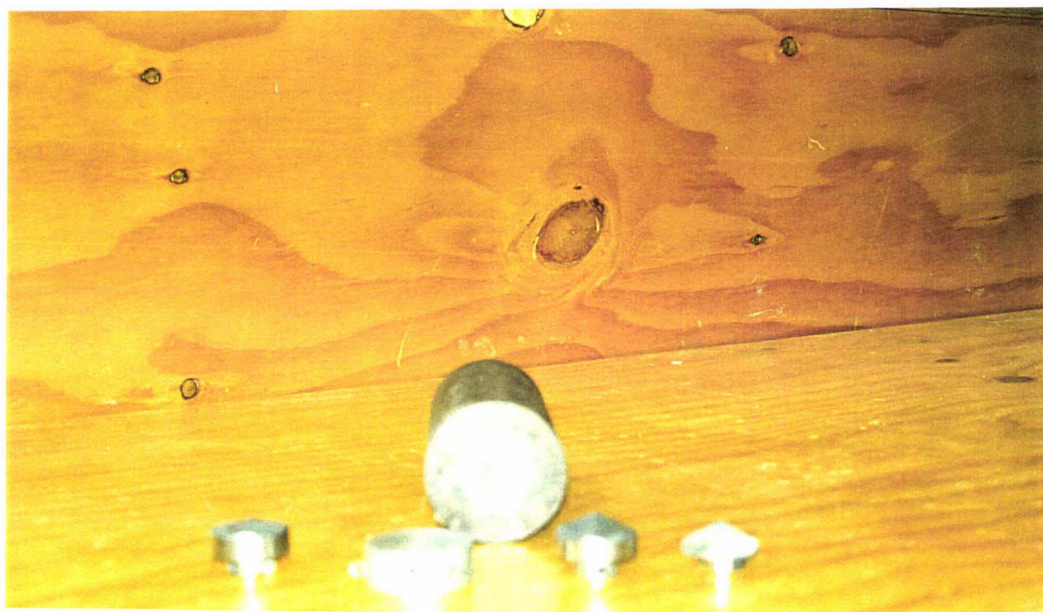
Figure 3.4 The different impact indenters selected for impact tests.
