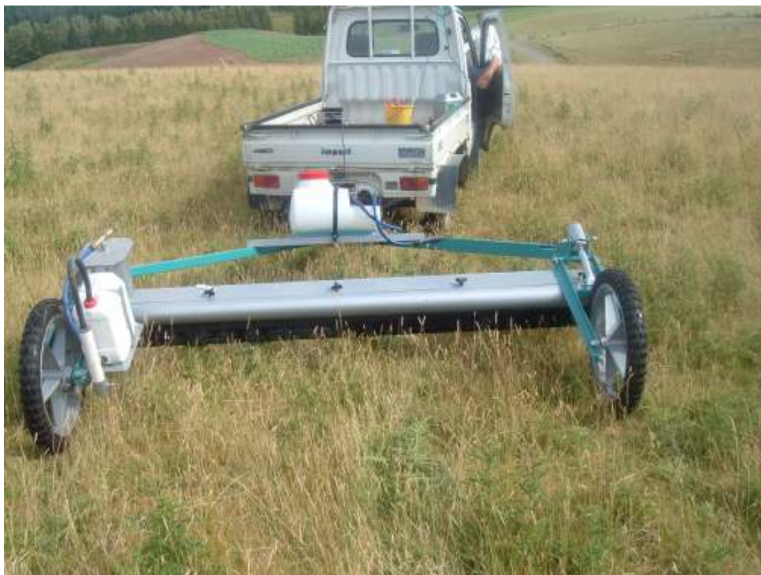
Plate 5.1 The rotary weed wiper (Rotowiper) used in the field trials
