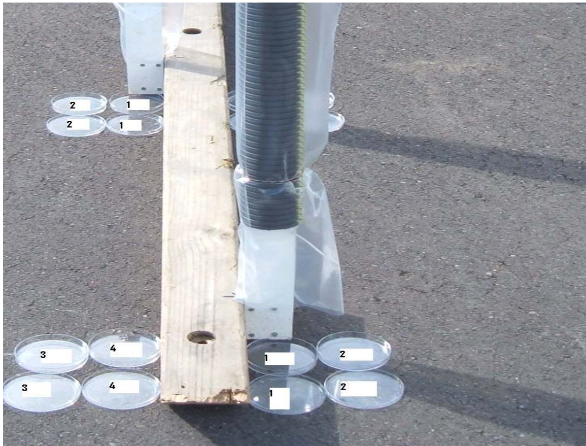
Plate 6.1 Arrangement of Petri dishes around the artificial weeds. The same number represents the dish and its lid.
