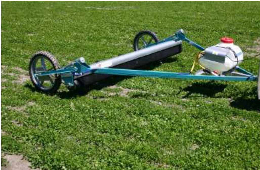
Plate 2.3 The Rotowiper similar to the one used in the trials (Source: www.rotoworks.co.nz )
