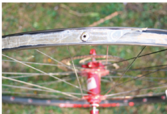
FIGURE 3. FRONT WHEEL WITH ONE 200G LEAD RIM STRIP IN PLACE.
