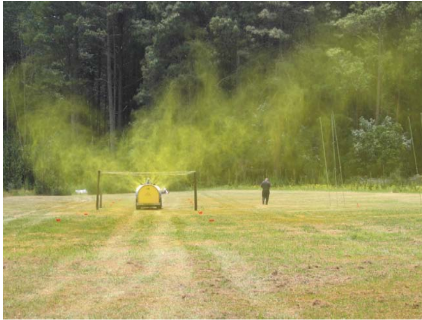
Figure 1.1: Spray released from an airblast sprayer. Photograph courtesy of Plant Protection Chemistry New Zealand.
