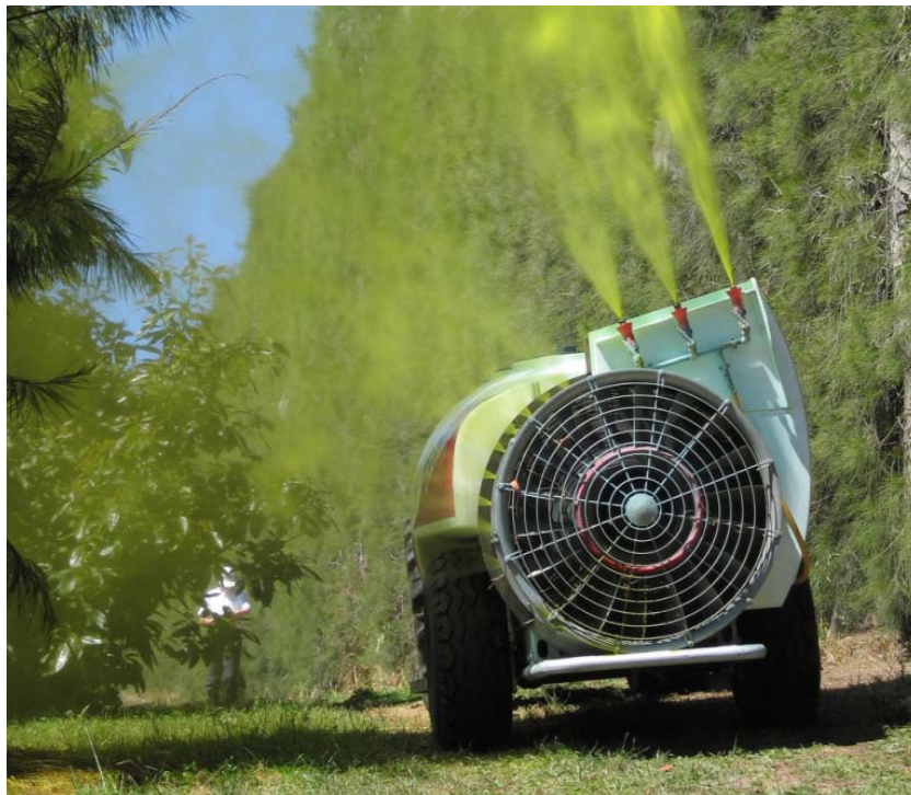
Figure 1.2: An airblast sprayer in an avocado orchard. Photograph courtesy of Plant Protection Chemistry New Zealand.
