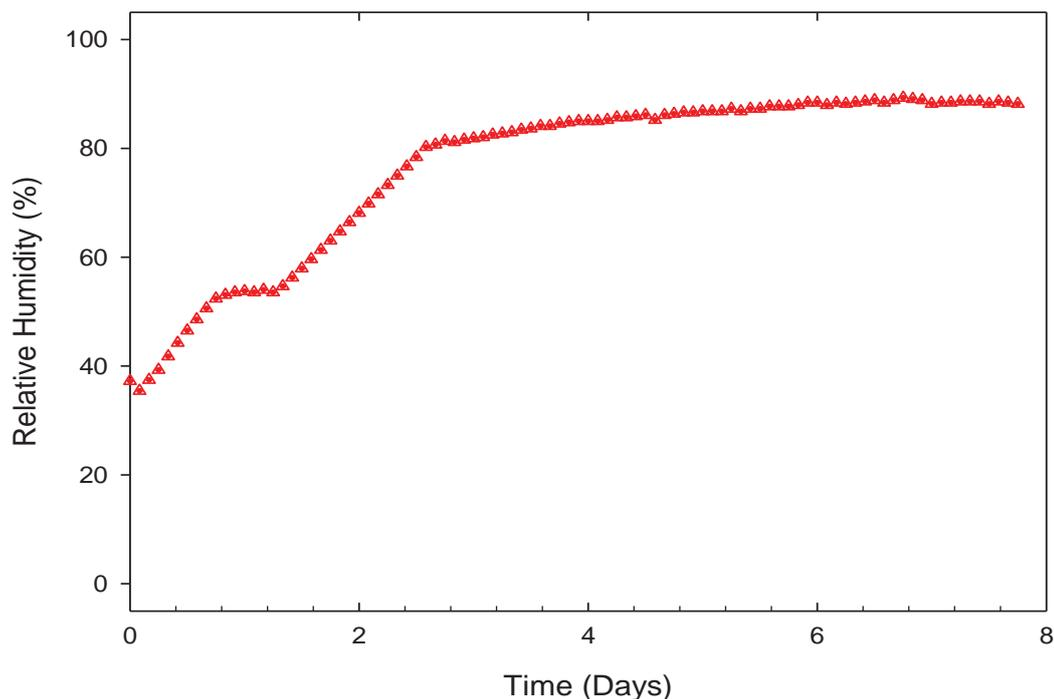
**Figure 7-5:** Results of extended experiment C (defined in Figure 7-3) (saturated salt solution – carvacrol oil – RH sensor) for the volatile flow through system (dry air flow rate 45mL/min; temperature 25°C).
