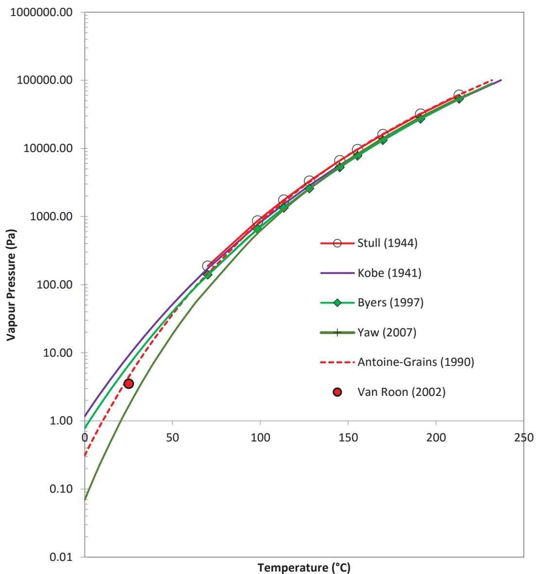
**Figure 7-2:** Comparison of carvacrol vapour pressure profiles derived from different sources. The experimental data was obtained from Stull (1947), Van Roon (2002) and Yaw (2007) and predicted results (solid lines) were derived from the Antoine equation while the dotted line (red) was derived from Antoine - Grains equation.
