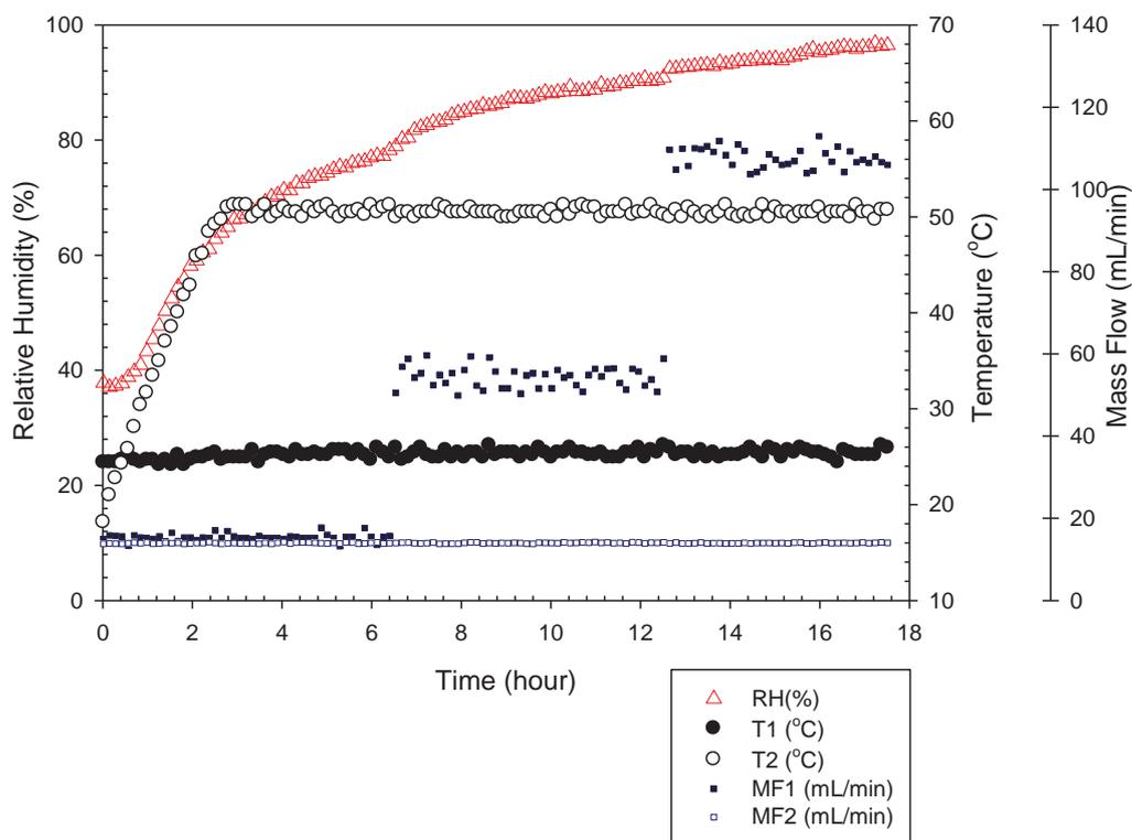
**Figure 7-16:** Experimental data to determine the effect of mass flow fraction against the relative humidity in the aluminium dish headspace. Legend represent  $F_{crv}:F_h$  ( $T_1 = 50^\circ\text{C}$ ,  $T_2 = 25^\circ\text{C}$ ,  $F_{crv}:F_h = 15:15$ ,  $15:50$  and  $15:100\text{mL} / \text{min}$ )
