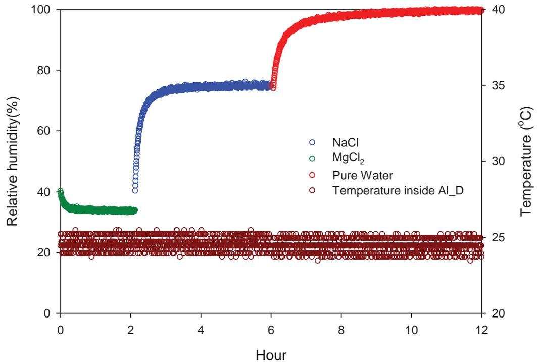
**Figure 7-14:** Example experimental data of bubble column operation with saturated salt solutions MgCl<sub>2</sub> (0 -2 h), NaCl<sub>2</sub> (2- 6 h) and pure water (6 h plus) at 25°C measured in the Aluminium Dish
