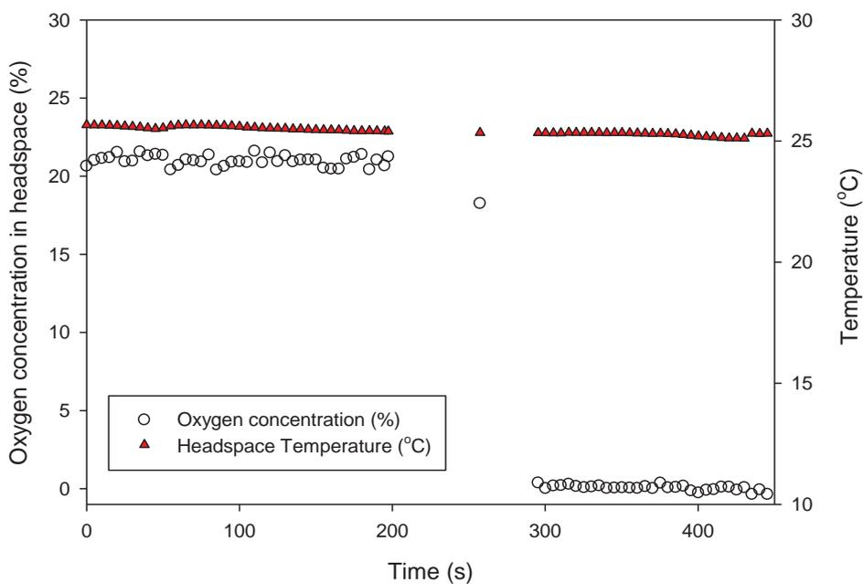
**Figure 5-5:** Plot of the two point calibration oxygen versus time in 120 mL Wheaton glass bottle headspace. The profiles show the oxygen concentration in the bottle headspace was up to 21.0% when dry air was introduced and plunged to 0.0% when dry air was replaced by pure nitrogen at time 300 seconds onwards
