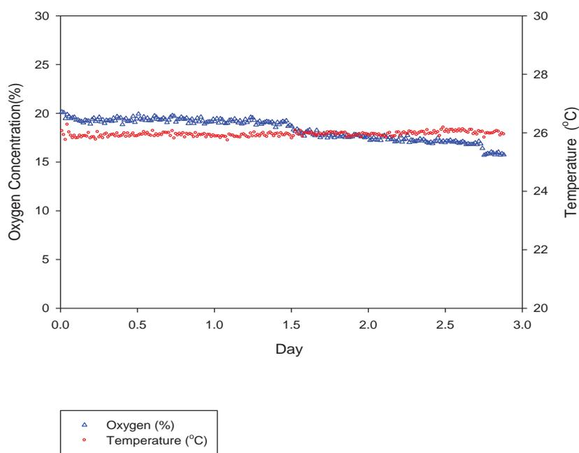
**Figure 5-6: Profiles oxygen concentration (%), temperature (°C) and Lifetime in the glass control Wheaton bottle (100mL headspace in potato dextrose agar incubated at  $25 \pm 1$  °C)**
