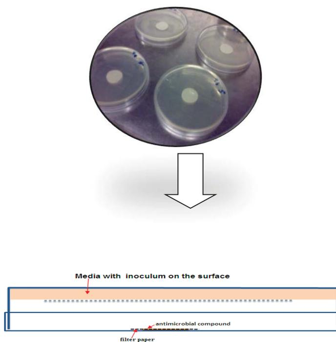
**Figure 3-3:** Illustration of Petri dish setup to determine the minimum inhibitory concentration in the vapour phase in this work based on the common micro-atmosphere method (Inverted Petri dish method).
