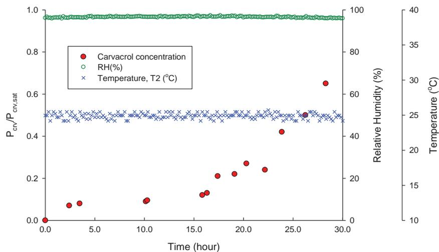
**Figure 7-19:** Plot of  $P_{cv}/P_{cv,sat}$ , Temperature (°C) and Relative Humidity against Time (hour) of the carvacrol volatile delivery system. ( $T_1$ , 50 °C, Water bath;  $T_2$ , 25 °C, Aluminium Dish); MFC1 = 100.0 mL/min; MFC2 = 14.0 mL/min).
