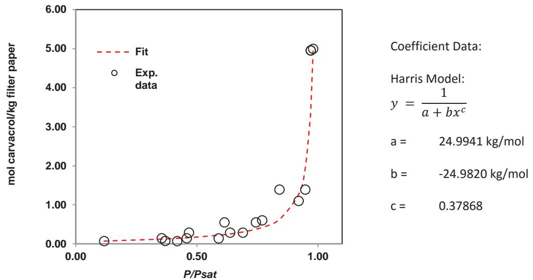
Figure 4-7: Experimental data and the curve-fitted equilibrium carvacrol concentration in the filter paper against carvacrol relative vapour pressure in the bottle headspace.
