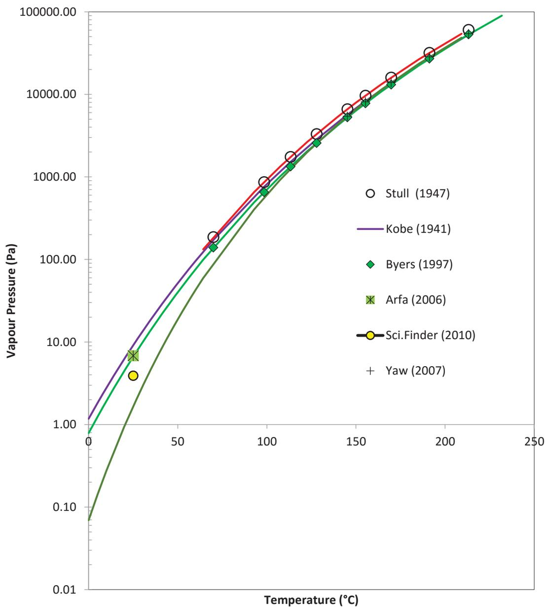
Figure 7-1: Comparison of carvacrol vapour pressure profiles derived from different sources of data. The experimental data was obtained from Stull (1947) and Yaw (2007) and predicted results (solid line) were derived from the fitted Antoine equations.
