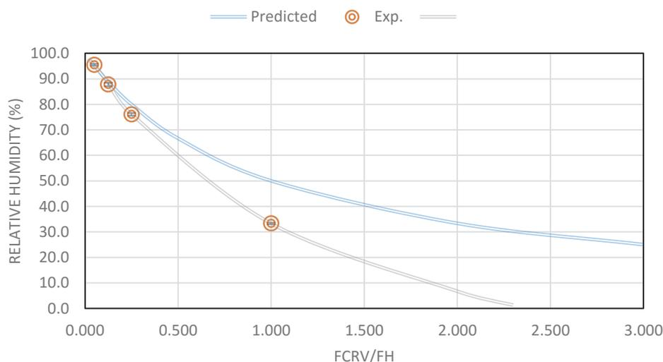
**Figure 7-17:** Experimental data of relative humidity (%) in the system (Aluminium Dish) at various ratios of  $F_{crv}$  and  $F_h$  and the predicted curve obtained by mass balance. Each data point was an average of 3 hours at equilibrium state (at frequency 20 seconds per data,  $N = 540$ ).
