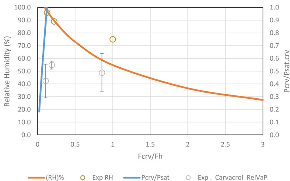
**Figure 7-18:** Experimental data of relative humidity (%) and relative carvacrol vapour pressure in the system (Aluminium Dish) at various ratios of  $F_{crv}/F_h$  (1(14:14), 0.22 (14:64), 0.13 (14:112) and the descriptive curve obtained by mass balance. Each point of carvacrol concentration was an average of three measurements and humidity experimental data was calculated as an average.  $T_1 = 50\text{ °C}$  and  $T_2, 25\text{ °C}$
