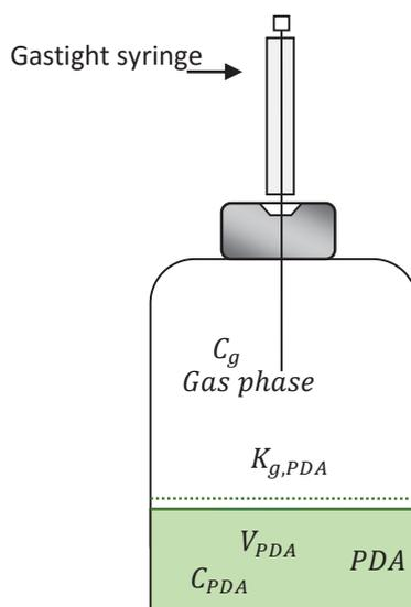
Figure 4-8: Illustration of sample and the phase in the Wheaton bottle as they relate to the partition coefficient
