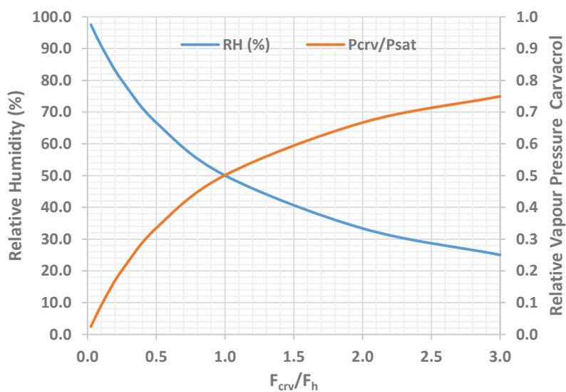
**Figure 7-8:** Theoretical mass balance of water and carvacrol vapour in the carvacrol delivery system at  $T_1$  and  $T_2 = 25^\circ\text{C}$ .
