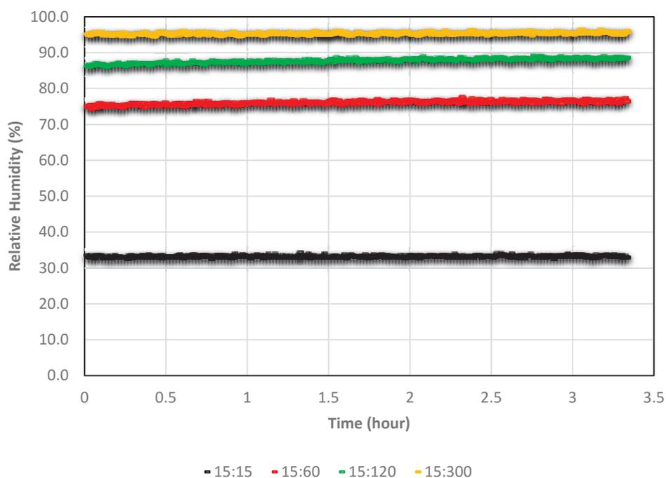
**Figure 7-15:** Effect of mass flow fraction against the relative humidity in the system headspace. Legend represent  $F_{crv}:F_h$  ( $T_1 = 25^\circ\text{C}$ ,  $T_2 = 25^\circ\text{C}$ ,  $F_{crv}:F_h = 15:15, 15:60, 15:120, 5:100$  mL / min) (note  $F_{crv}$  was effectively dry air as no carvacrol oil was present in the bubble column).
