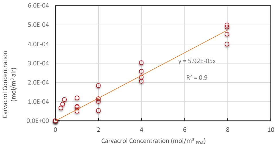
**Figure 4-9:** Carvacrol partitioning, (mol/m³ air) vs. (mol/m³ PDA). Measurement of the gas phase in the sample vials was performed after the samples were stored at 25°C overnight. (Direct Method: Vapour Phase Calibration method)
