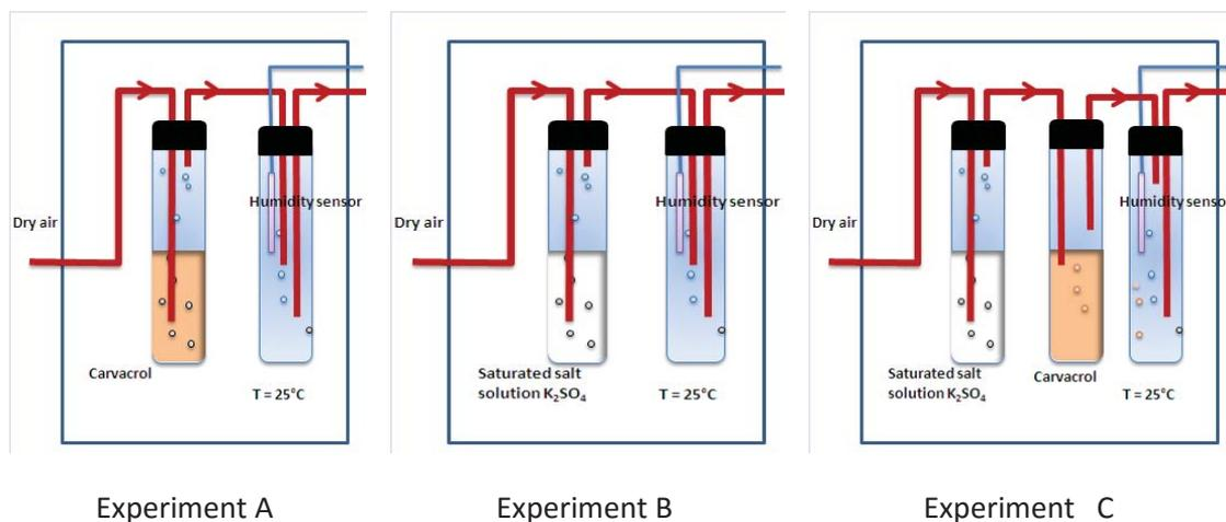
**Figure 7-3: Illustration of experiments conducted to get the required relative humidity in flow through system.**
