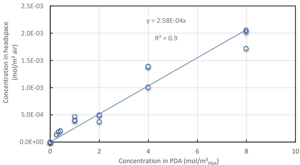
**Figure 4-10:** Thymol partitioning (mol/m³ air) vs. (mol/m³ PDA). Measurement of the gas phase in the sample vials were performed after the samples were stored at 25°C overnight (Direct Method: Vapour Phase Calibration method).
