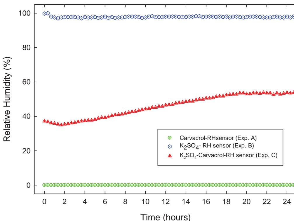
**Figure 7-4:** Results of an experiment for the volatile flow through experimental setups A, B and C defined in Figure 7-3 (dry air flow rate 45mL/min; Temperature 25°C).
