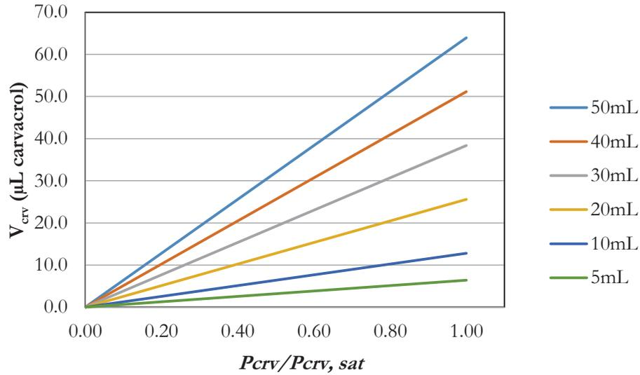
**Figure 5-1:** Profiles carvacrol volume ( $\mu\text{L}$ ) against carvacrol relative vapour pressure at a different volume of PDA in 120 mL Wheaton bottle.
