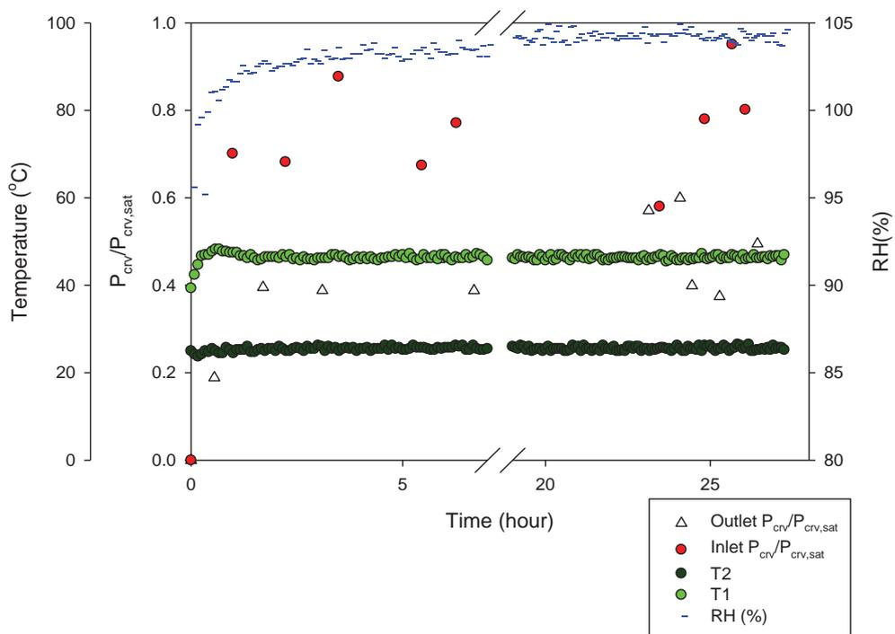
Figure 7-20: Carvacrol concentration at sampling point 1(SP1, inlet) and in the sampling point (SP2, outlet) of the system delivery
