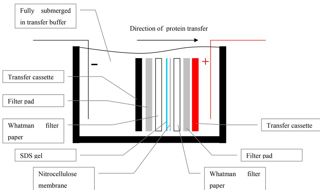
**Figure 84: Western blot apparatus set-up of electro blotting sandwich**
