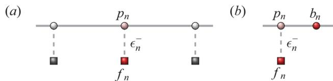
Fig. 2: (Color online) Detangled Fano lattices. (a) Cross-stitch lattice from fig. 1(a) detangled with eqs. (4), (5). Horizontal couplings are of strength 2, and vertical couplings follow  $\epsilon_n^-$ . (b) Tunable diamond chain from fig. 1(b).
