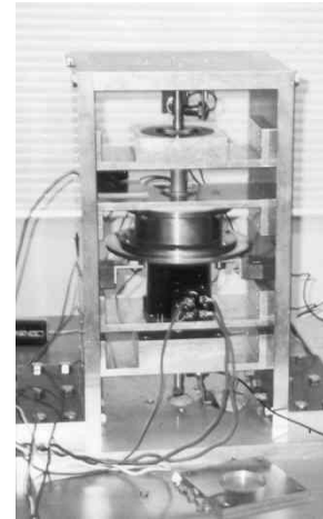
Fig. 1. Magnetic bearing for vertical shaft machine.
