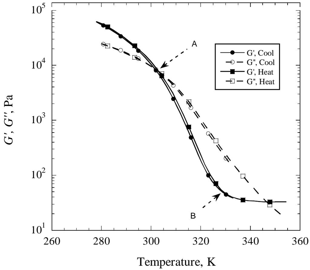
Figure 5 – Gelation and softening temperatures of sodium caseinate dispersions
