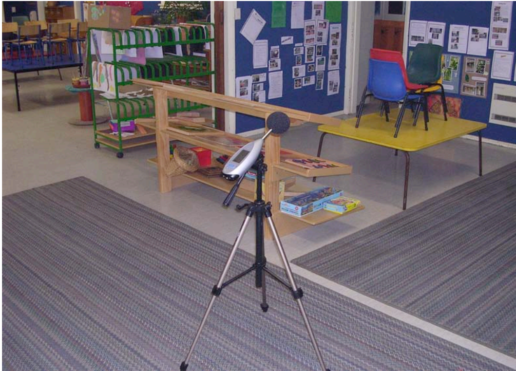
Figure 7-9 Measurement of reverberation times ( T_{60} ) with Solo Master sound level meter.
