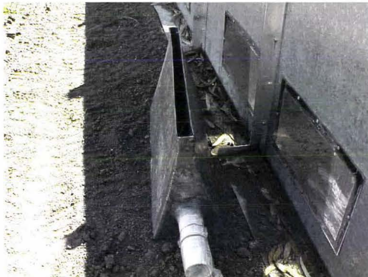
Figure 2.6.3: The Nickling sediment sampler used for the Hawke's Bay research
