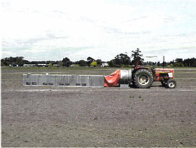
Figure 2.6.1: The Lincoln University Wind Tunnel (LUWT) set up on a Pakipaki plot
