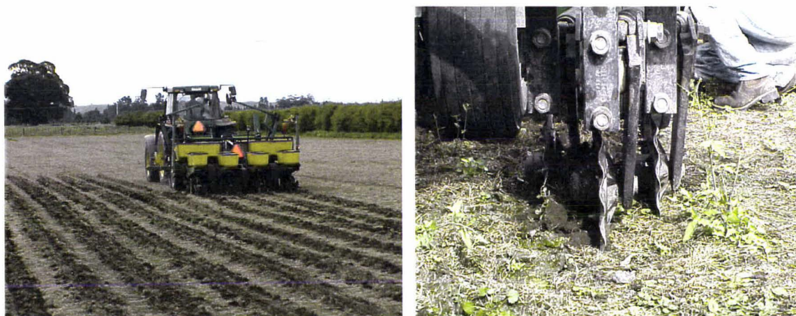
Figure 3.2.1: The modified Great Plains corn planter used for the minimum tillage treatment: left – preparing trial plot; right – the front set of discs on the planter.
