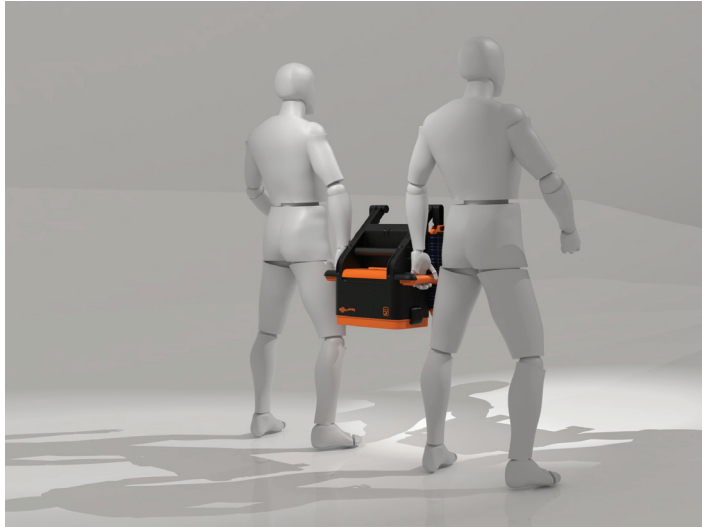
Figure 138. Recommended two man lift
