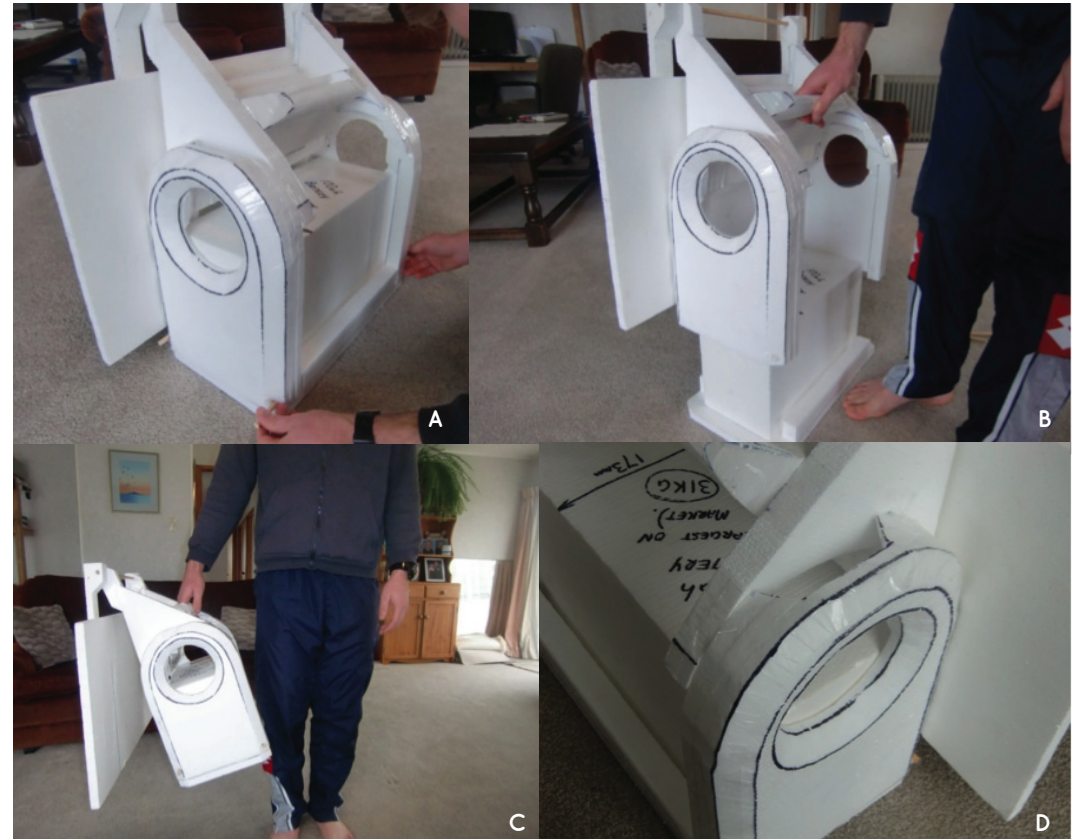
Figure 92. A) Pulling pins to release the body from the base. B) Removing body for complete access to battery. C) Identifying balance issue. D) Handle detailing
