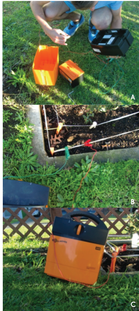
Figure 29. A) Opening Gallagher B40 to investigate the inside components. B) The participant has attached the grounding cable to the fence (common misunderstanding). C) Lid has been put on incorrectly. The reverse clip prevents extraction of the lid in this position
