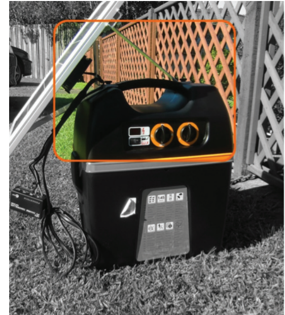
Figure 88. Gallagher Powerbox solar panel issue (handle obstruction)
