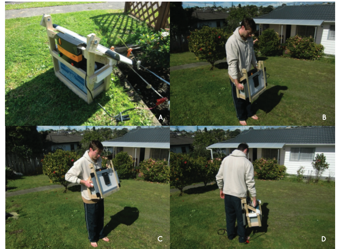
Figure 104. A) All components fitted and connected to the fence. B) Two-hand Lifting – Arms straight. C) Two-hand Lifting – Lifted to stomach height, arms bent. D) Single handle lift – Straight arm, one sided weight
