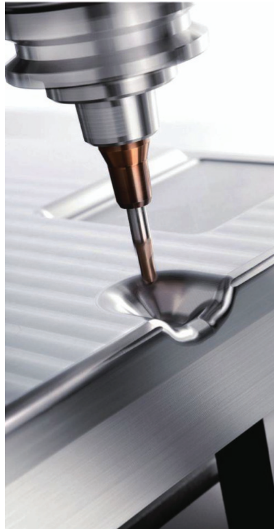
Figure 17. Machining an injection moulding tool
