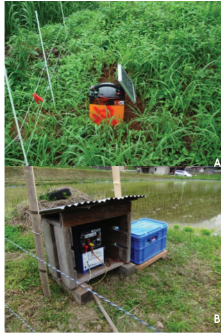
Figure 33. A) Gallagher B40 working amongst long grass. B) Permanent energizer setup installed in a small shelter to protect from the elements (Japan)
