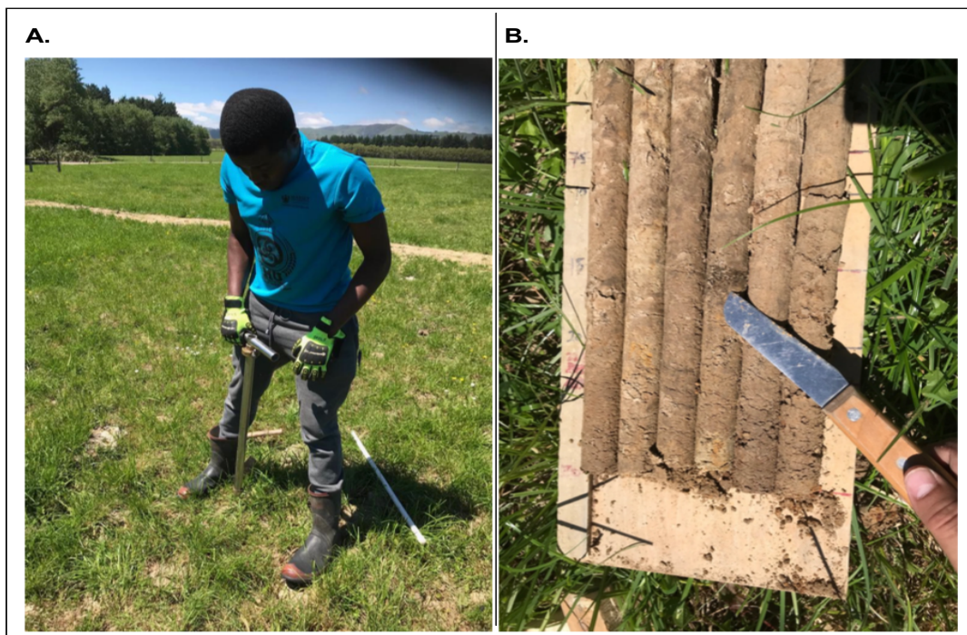
Figure 3.3. Sampling activity at Field trial 3 (Massey University's No.4 dairy farm-paddock 50) on 14 November 2018, about 8 months after the new grass was established. A) soil coring to 30 cm depth using a percussion corer B) soil core columns arranged for slicing into representative depth intervals of 0-7.5, 7.5-15, 15-22.5 and 22.5-30 cm.
