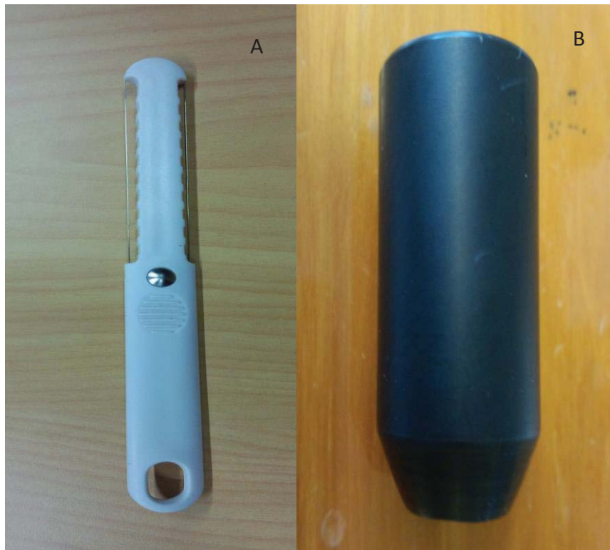
Figure 9 - 2 Cheese slicer (A) and 20 mm cork borer (B)
