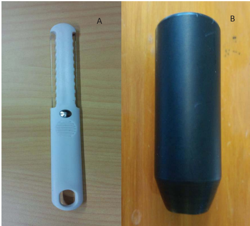
Figure 5 - 2 Cheese slicer (A) and 20 mm cork borer (B)
