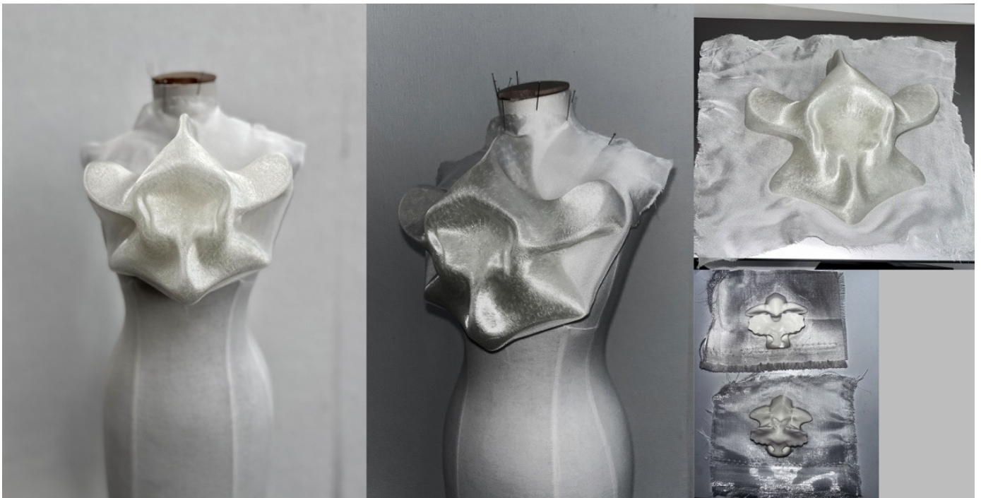
Figure 4.27 FDM-printed structural samples integrated with silk fabric (author's documentation photograph).
