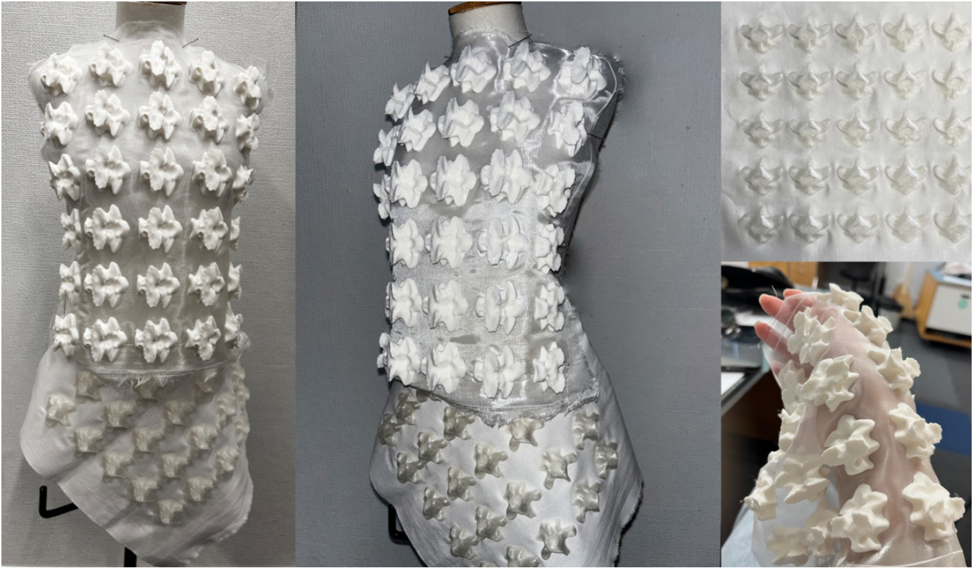
Figure 4.28 Repeated-printing strategy applied to silk and cotton fabrics for flexible structural attachment (author's documentation photograph).
