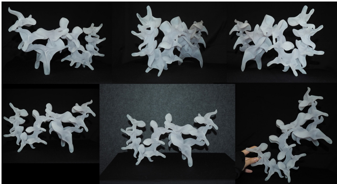
Figure 4.30 Semi-transparent resin FloraCore prototype printed using Kings SLA 400 with post-processing surface refinement (author's documentation photograph).
