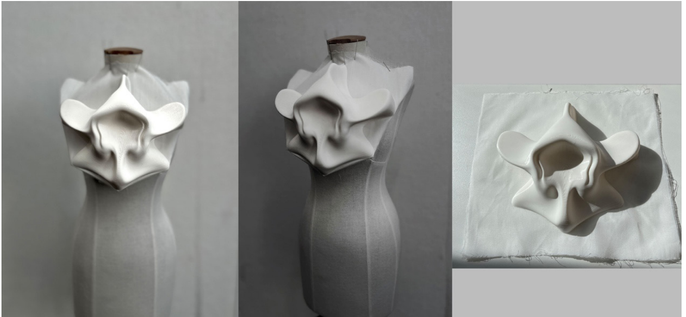
Figure 4.26 FDM-printed structural samples integrated with cotton fabric (author's documentation photograph).
