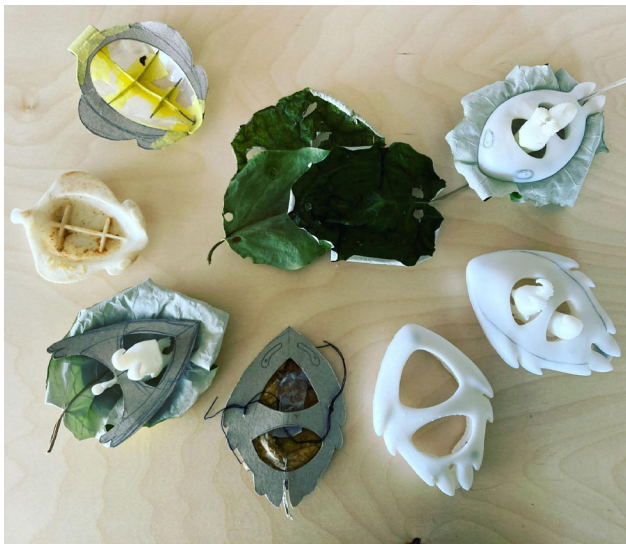
Figure 73: Cycle of prototypes for the Leafy Boat character, showing design development and integration through iterative design testing/trialling cycles. Rangiora leaves at centre, then clockwise from top left: cardboard model, quick 3D print, cardboard models with Rangiora leaves, resolved 3D print models with Rangiora leaves. Prototypes and photo by Tanya Marriott.
