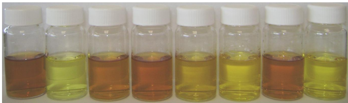
Figure 23. IPA solutions of 1 in the presence of the acids studied in this chapter. From left to right the solutions are; 1 only, 1 +HCl, 1 +HBr, 1 +HNO 3 , 1 +HBF 4 , 1 +HClO 4 , 1 +H 3 PO 4 and 1 +SO 4 . Concentration of 1 is 360 \mu\text{mol L}^{-1} and acids are present at 100 equivalents.
