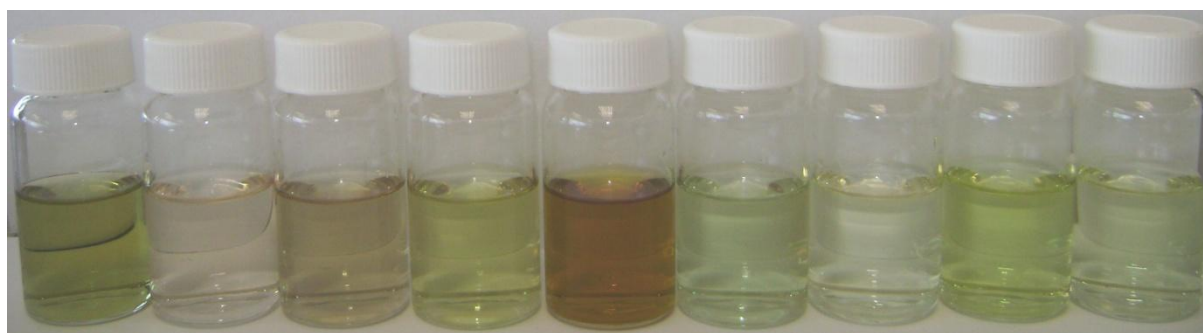
Figure 39. DCE-IPA solutions of 2 in the presence of the acids studied in this chapter. From left to right the solutions are; 2 only, 2 +HCl, 2 +HBr, 2 +HNO 3 , 2 +HI, 2 +HBF 4 , 2 +HClO 4 , 2 +H 3 PO 4 and 2 +H 2 SO 4 . The concentration of 2 is 349 \mu\text{mol L}^{-1} and acids are present at 100 equivalents.
