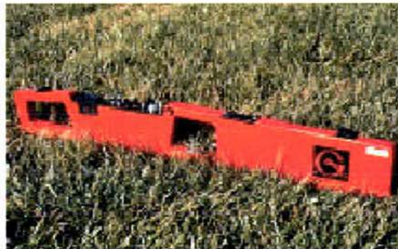
Figure 4.2 Non-contact EM38 sensor used to measure soil electrical conductivity. Source: USDA-ARS Photo Gallery.
