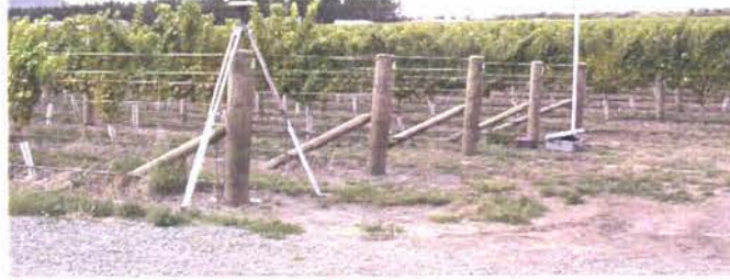
Figure 4.4 RTK-DGPS base station installed at the Rarangi Vineyard.
