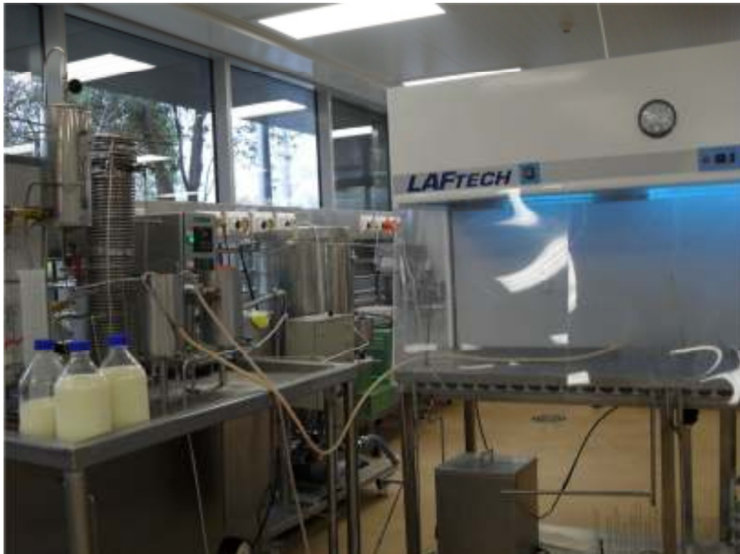
Figure 3.2: Indirect UHT plant (Alfa Laval) use for UHT treatment for yoghurt milk base
